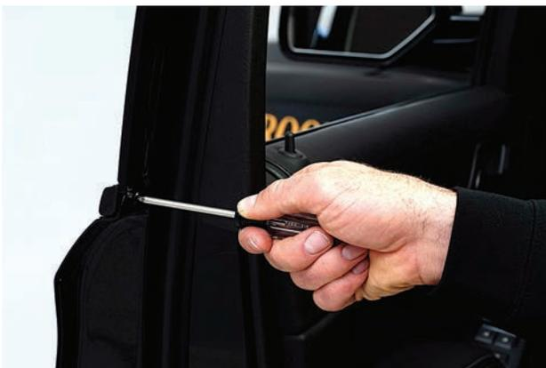
▲ Figure 5. Removing outer window weatherstrip screw
