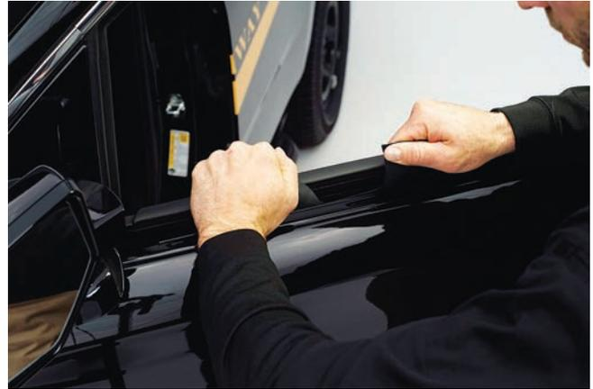
▲ Figure 9. Gripping and sliding the ballistic door panel forward into place.
