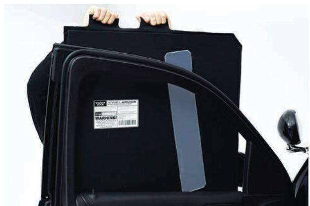
▲ Figure 7. Inserting ballistic panel into door with anti-abrasion panels facing vehicle interior
