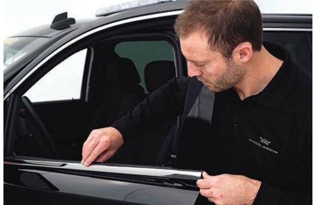
▲ Figure 6. Removing outer window weatherstrip
