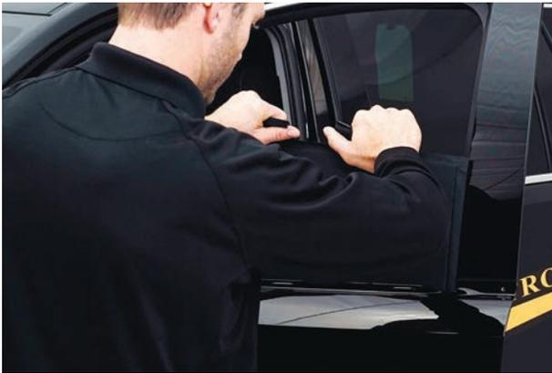
▲ Figure 8. Holding ballistic door panel against window glass while leaning back
