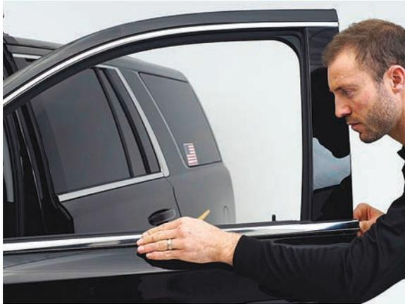
▲ Figure 11. Reinstalling outer window weatherstrip
