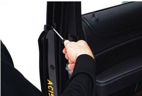
▲ Figure 12. Replacing outer window weatherstrip screw
