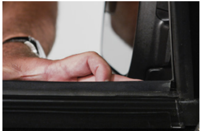
▲ Figure 20. Proper alignment of nylon fold with window frame
