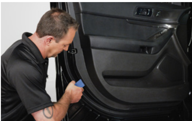
▲ Figure 11. Prying open the vehicle interior door trim panel
