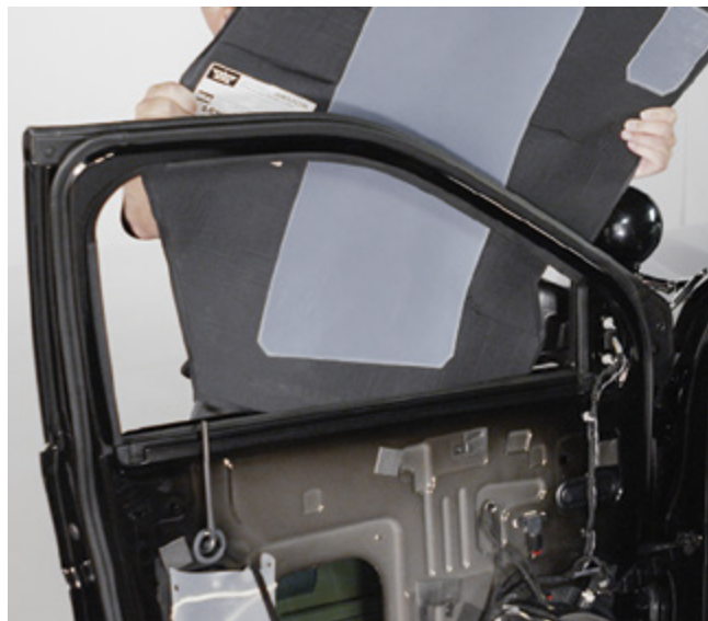
▲ Figure 18. Inserting the panel into the door
