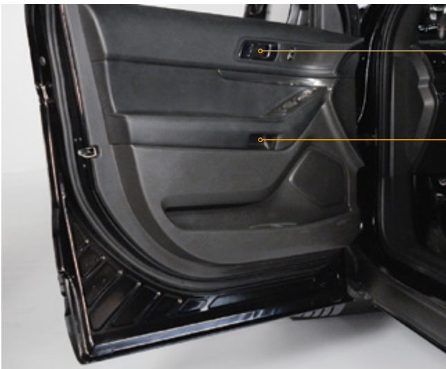
▲ Figure 9. Trim cover and bolt locations
