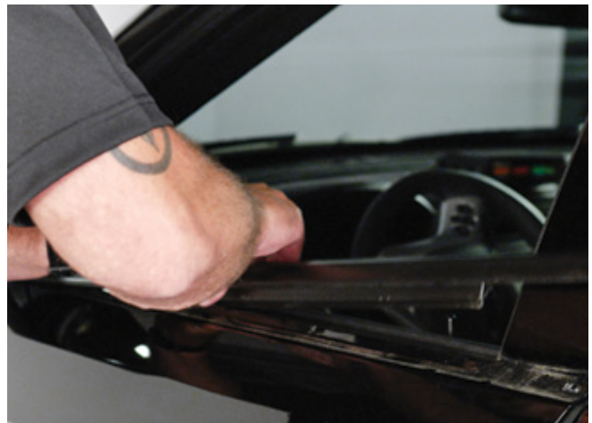
▲ Figure 7. Removing the window trim
