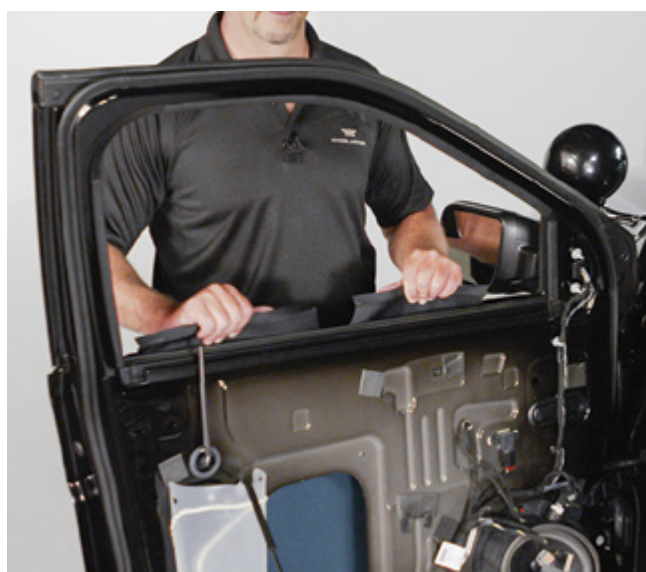
▲ Figure 19. Gripping ballistic door panel's top-edge nylon folds
