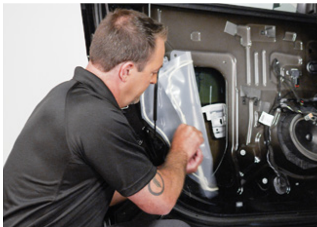
▲ Figure 14. Peeling back the moisture barrier to expose the window regulator bolt
