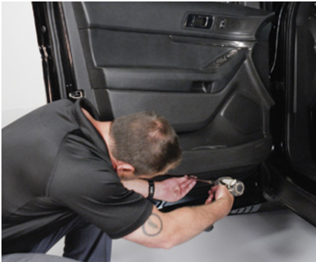
▲ Figure 8. Removing 7 mm panel mounting bolts
