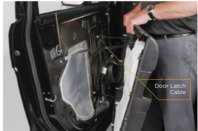
▲ Figure 12. Location of the door latch cable
