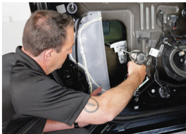
▲ Figure 15. Replacing the factory-installed window regulator bolt located behind the moisture barrier with the supplied replacement bolt
