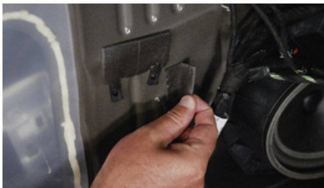
▲ Figure 16. Removing black foam cover to expose window regulator bolt access hole
