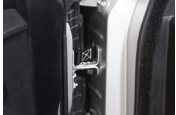
▲ Figure 19. Proper placement of the secured check strap.
