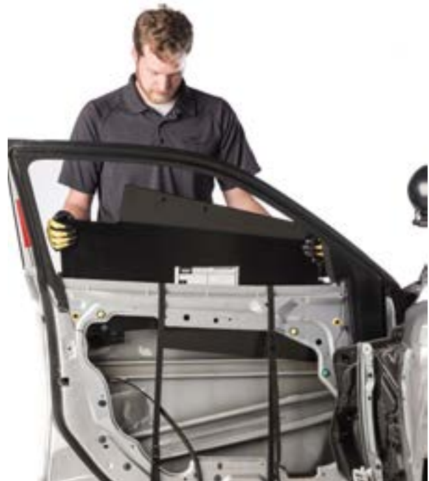
▲ Figure 39. Using the cradle created by the installation straps to lower the armor into the door.
