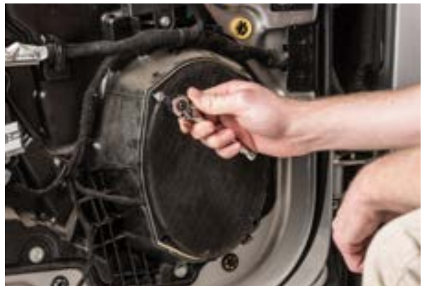
▲ Figure 30. Removing the speaker screws.
