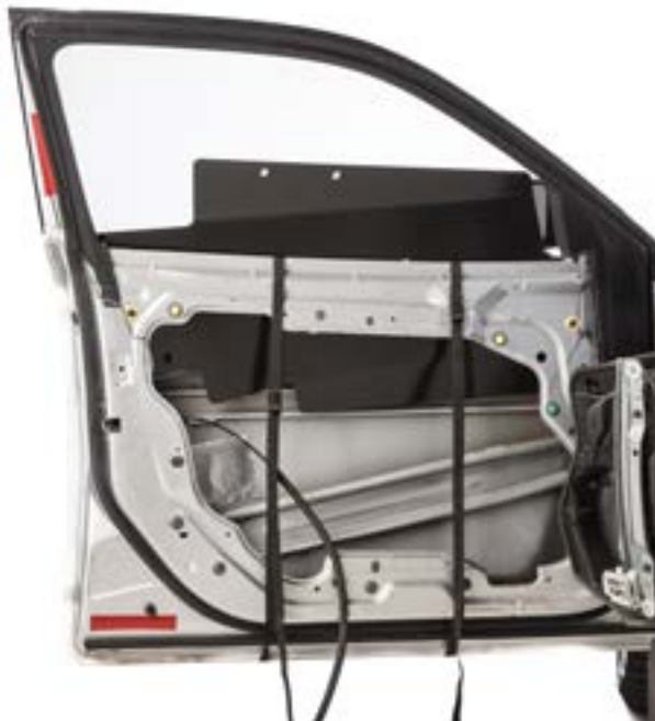
▲ Figure 40. Proper placement of the armor installed \frac{3}{4} of the way into the door.
