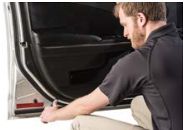
▲ Figure 28. Prying the door panel away from the door skin.
