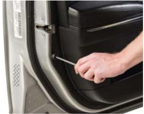
▲ Figure 27. Removing screw at bottom edge of the door panel.
