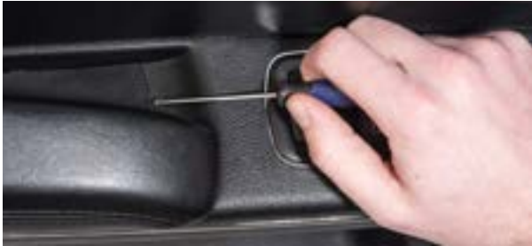
▲ Figure 25. Removing the armrest pocket trim cover.
