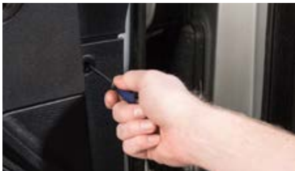
▲ Figure 26. Removing the fastener at the inner edge of the door panel.
