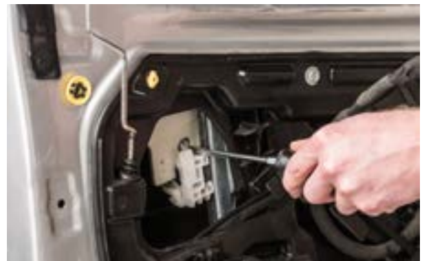
▲ Figure 33. Releasing the back window clip.
