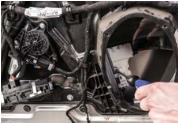
▲ Figure 31. Releasing the front window clip.
