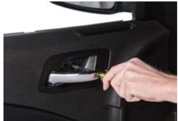
▲ Figure 24. Removing the interior door handle screw.
