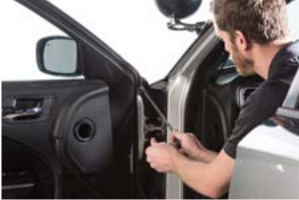
▲ Figure 20. Removing the front window weatherstrip screw.
