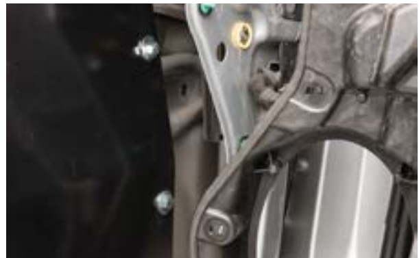
▲ Figure 46. The front, bottom crash bar bracket loosely installed.
