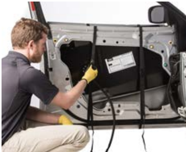
▲ Figure 45. Lowering the armor into the door using the installation straps.
