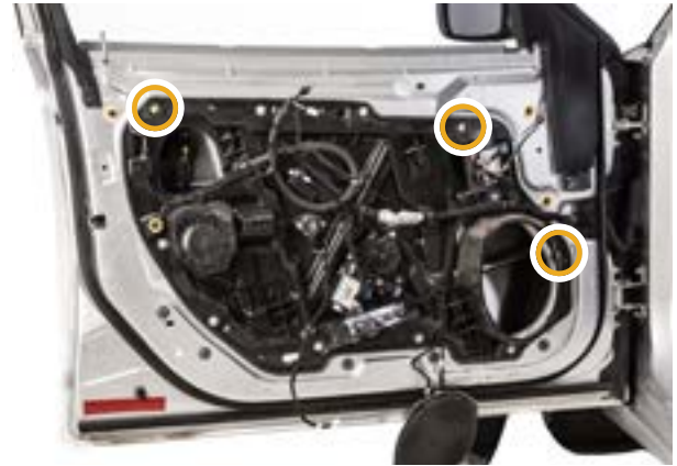
▲ Figure 36. Location of the clips around the inner door panel.
