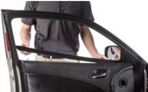
▲ Figure 22. Removing the outer window weatherstrip.
