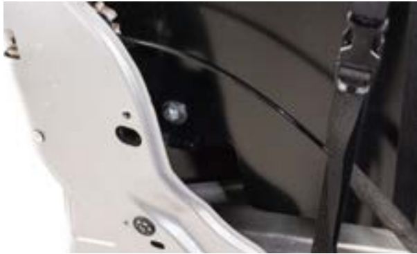
▲ Figure 44. The back crash bar bracket loosely installed.
