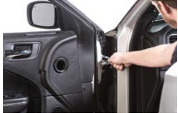
▲ Figure 18. Removing the upper door hinge bolt and nut.
