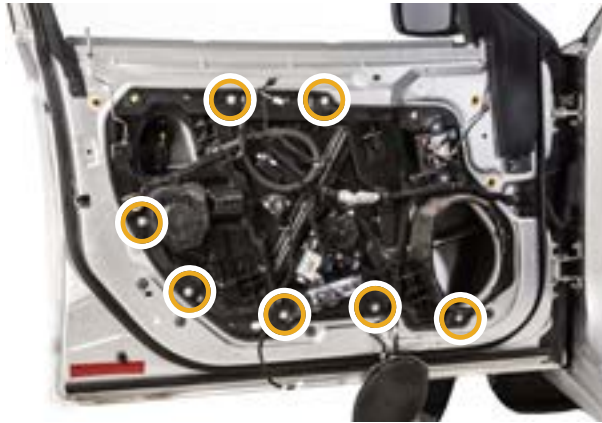
▲ Figure 34. Location of the bolts around the inner door panel.
