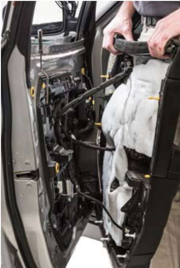
▲ Figure 29. Tilting the door panel away from the door skin.
