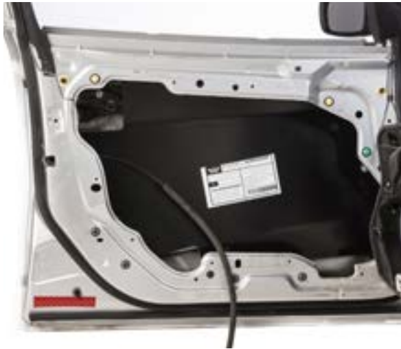
▲ Figure 47. The armor in its final position inside the door.
