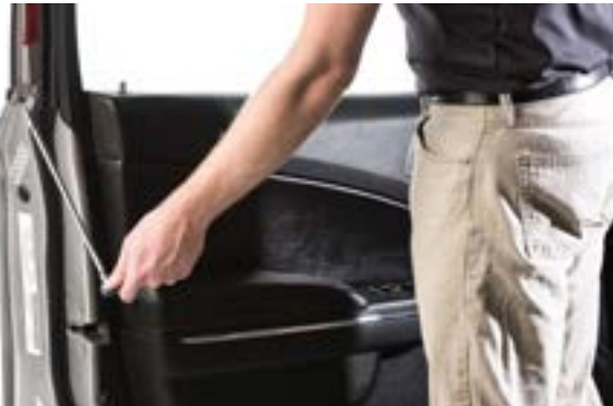
▲ Figure 21. Removing the back window weatherstrip screw.
