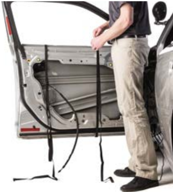
▲ Figure 37. Looping the installation straps around the door.
