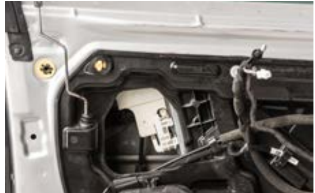
▲ Figure 32. Location of the window regulator access panel.
