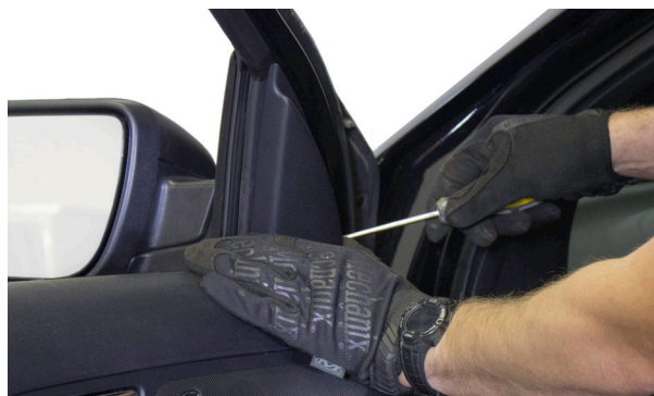
▲ Figure 26. Prying the side mirror interior trim panel away from the door.
