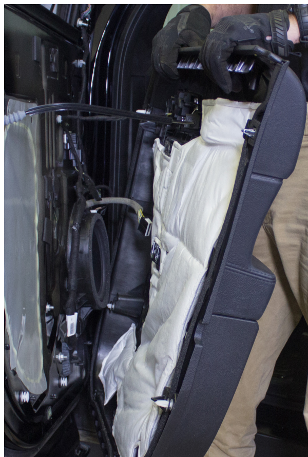
▲ Figure 28. Tilting the door panel away from the door skin.
