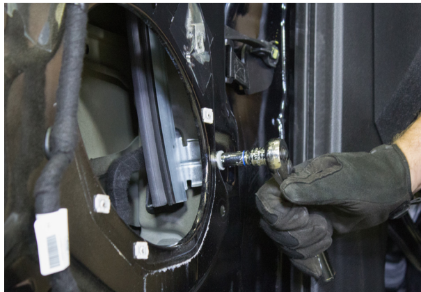
▲ Figure 32. Removing the window track bolt.
