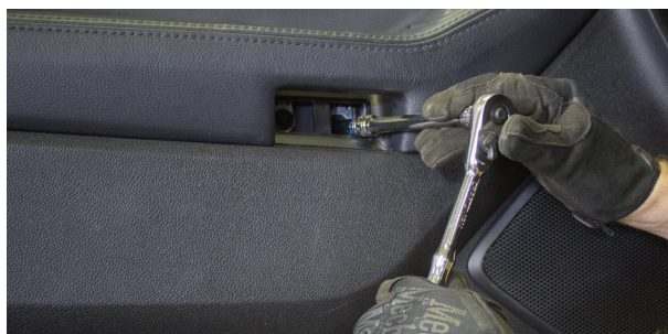
▲ Figure 23. Removing the armrest pocket bolts.
