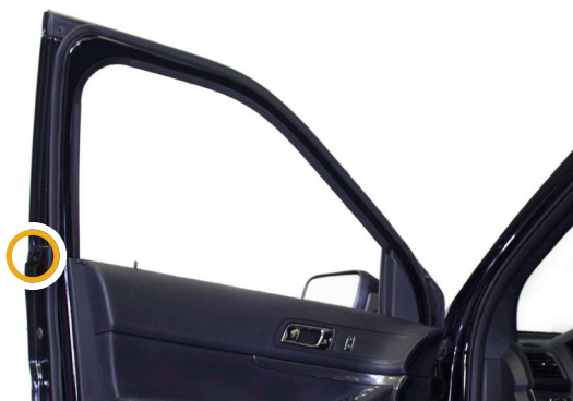
▲ Figure 18. Removing the back window weatherstrip screw.
