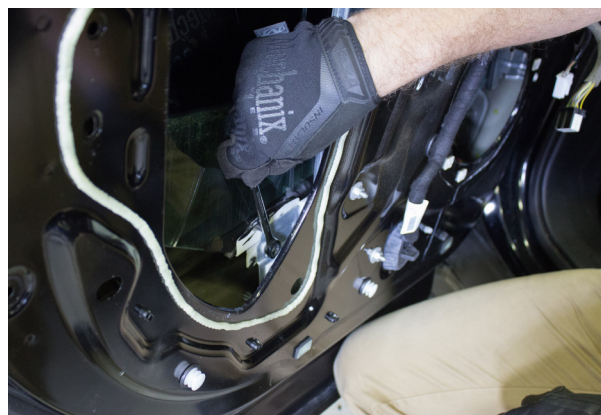
▲ Figure 30. Removing the window mounting bolts.
