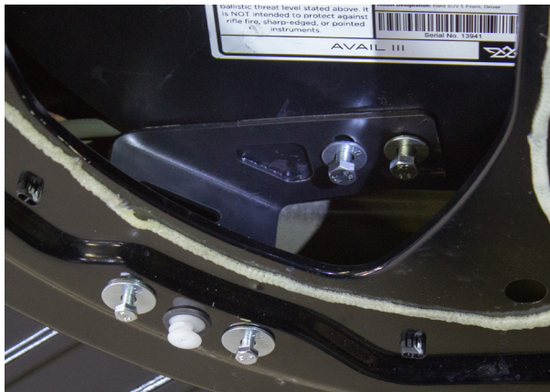
▲ Figure 45. Lower mounting bracket loosely installed.
