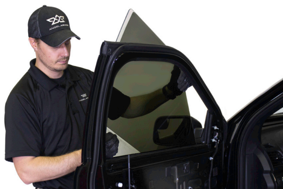
▲ Figure 31. Removing the window glass.
