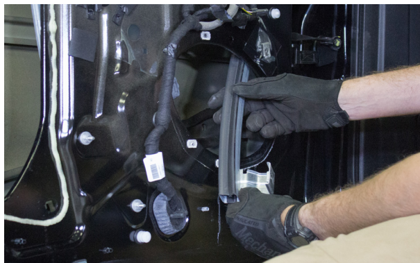
▲ Figure 33. Removing the window track.
