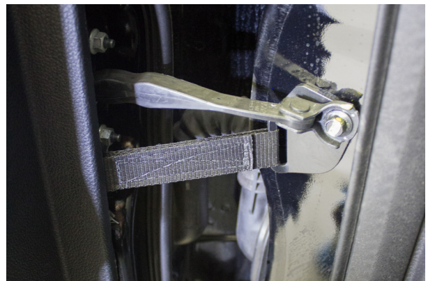
▲ Figure 17. Proper placement of the secured check straps.
