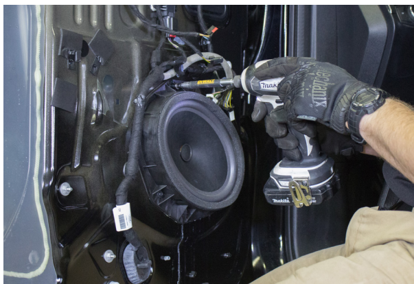
▲ Figure 29. Removing the speaker screws.
