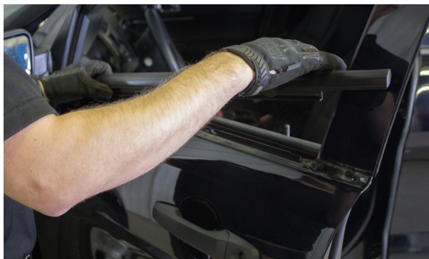
▲ Figure 19. Removing the outer window weatherstrip.
