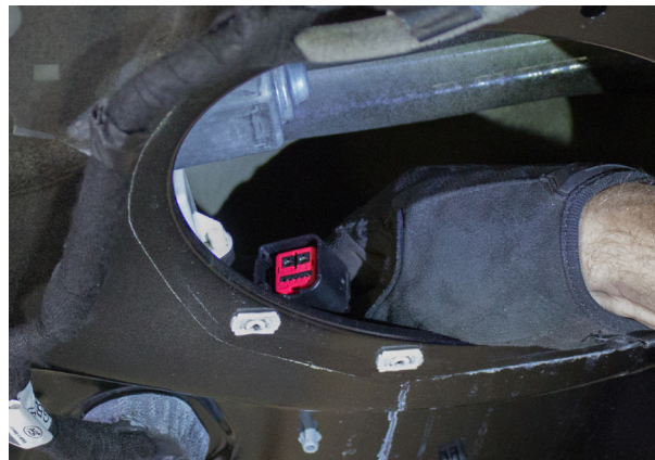
▲ Figure 34. Disconnecting window regulator wiring harness.
