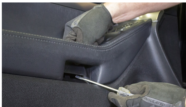
▲ Figure 22. Removing the armrest pocket trim cover.
