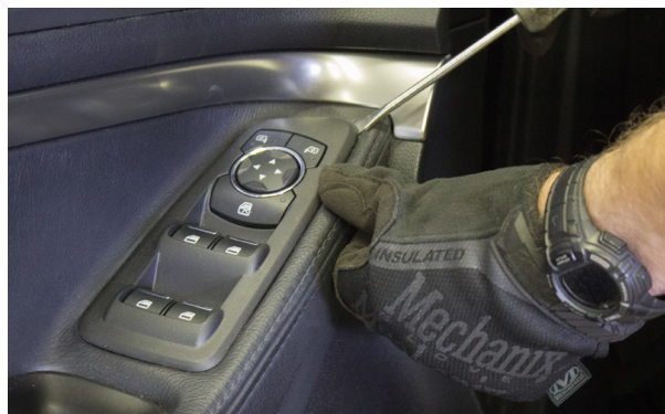
▲ Figure 25. Prying up the window control panel.
