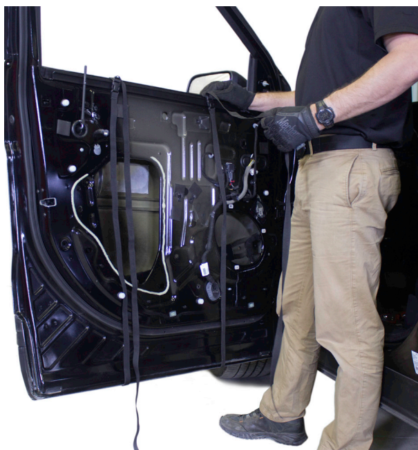
▲ Figure 39. Looping the installation straps around the door.
