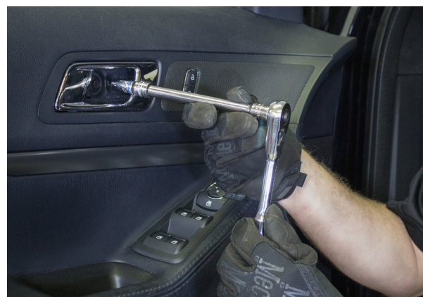
▲ Figure 21. Removing the interior door handle bolt.
