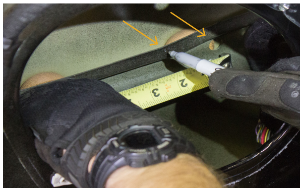
▲ Figure 36. Marking 2 inches toward the rear of the vehicle from the center of the forward crash bar hole.
