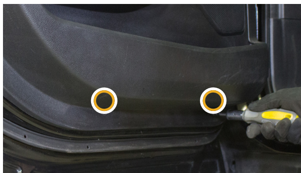
▲ Figure 24. Removing the door panel bolts.
