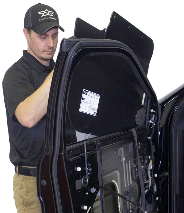
▲ Figure 41. Placing the armor into the door.
