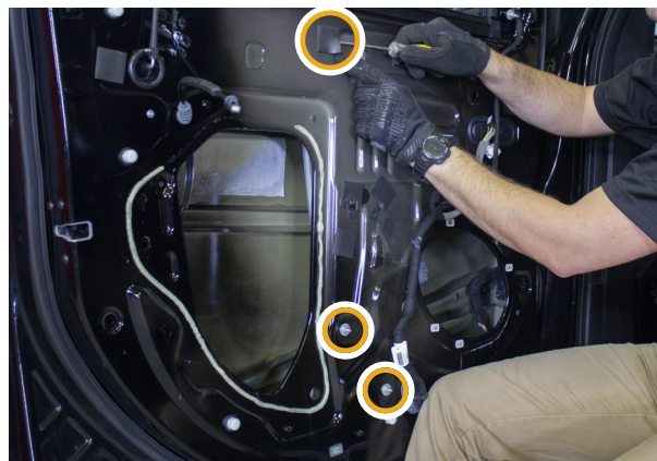
▲ Figure 35. Location of the three window regulator fasteners.
