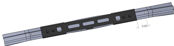
▲ Figure 37. Rendering of the Crash Bar Mounting bracket showing location on crash bar.
