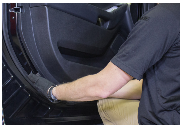
▲ Figure 27. Prying the door panel away from the door skin.
