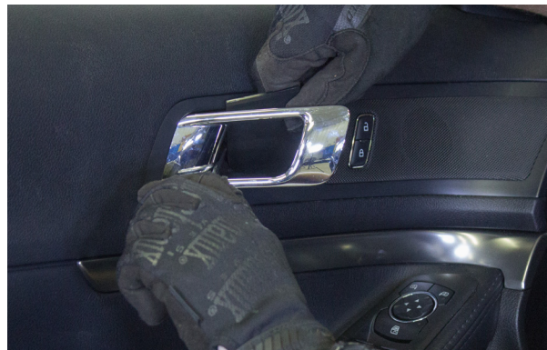
▲ Figure 20. Remove the interior door handle trim cover.
