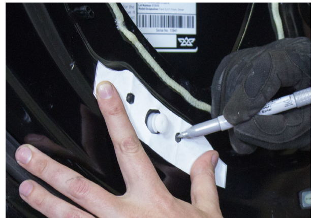
▲ Figure 44. Marking the hole locations using the template provided (appended to the end of this guide).
