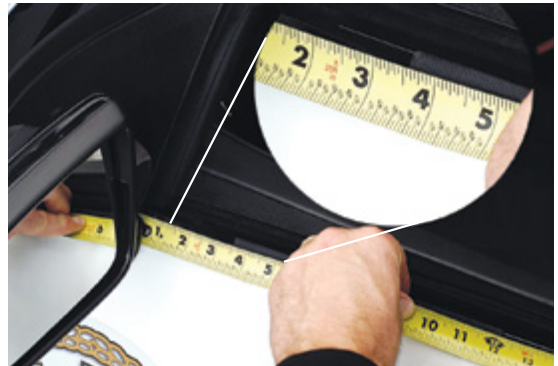
▲ Figure 28. Proper measurement from the front edge of the nylon to the vertical edge of the window frame
