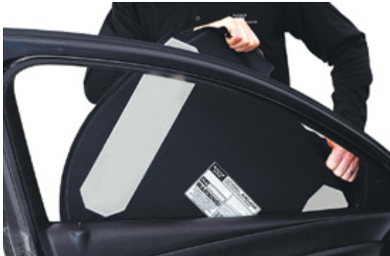
▲ Figure 26. Rotating the back edge of the ballistic panel into the door
