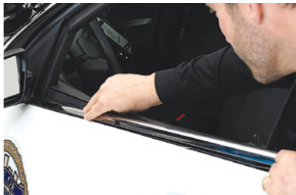
▲ Figure 31. Pressing down on the entire length of the weatherstrip
