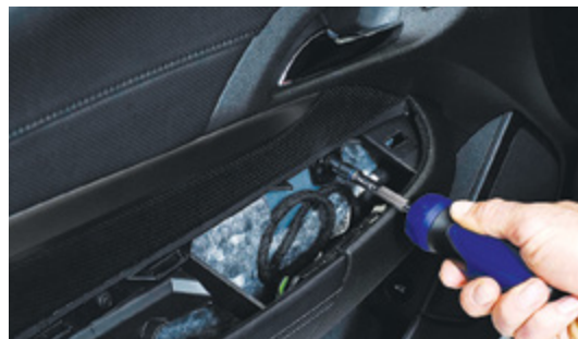
▲ Figure 15. Removing the 10 mm bolt from behind the window control panel
