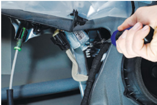
▲ Figure 22. Replacing factory installed window bolt with shorter bolt included in the installation kit
