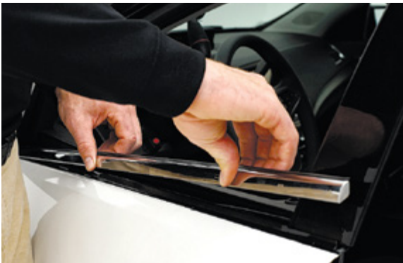
▲ Figure 24. Removing outer window weatherstrip
