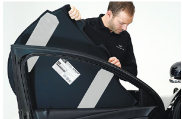
▲ Figure 25. Inserting the ballistic panel into the door at an angle
