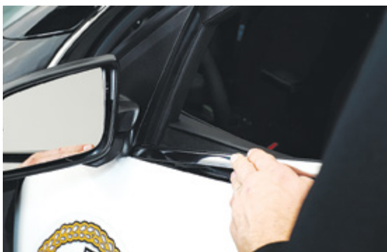
▲ Figure 30. Reinstalling weatherstrip under rear-view mirror
