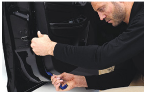
▲ Figure 17. Prying open the interior vehicle door panel
