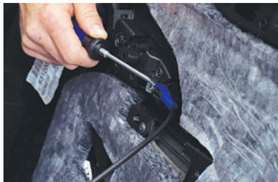
▲ Figure 20. Disconnecting door latch cable
