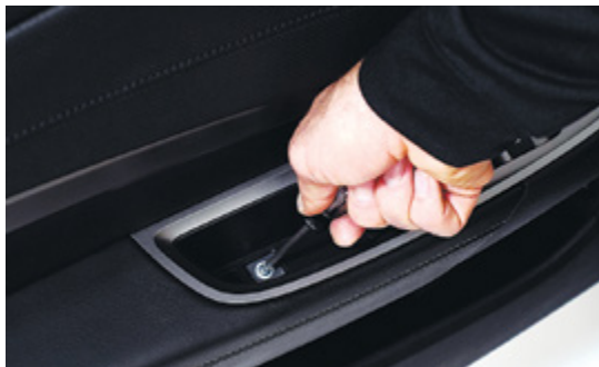
▲ Figure 12. Removing the Phillips screw from the arm rest pocket
