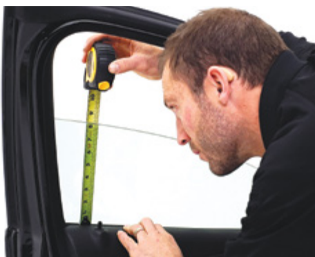
▲ Figure 7. Adjusting the window glass to 8.25 inches
