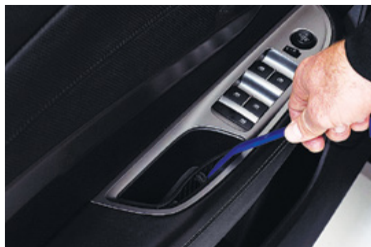
▲ Figure 11. Removing the rubber trim cover from the arm rest pocket
