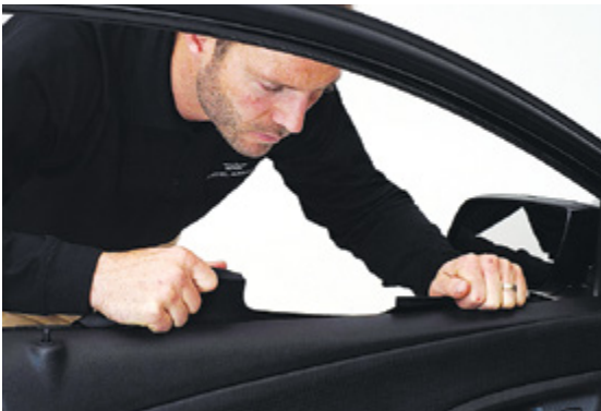
▲ Figure 27. Gripping ballistic door panel's top-edge nylon folds
