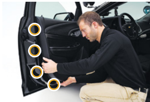
▲ Figure 16. Approximate locations of the interior door trim retainers
