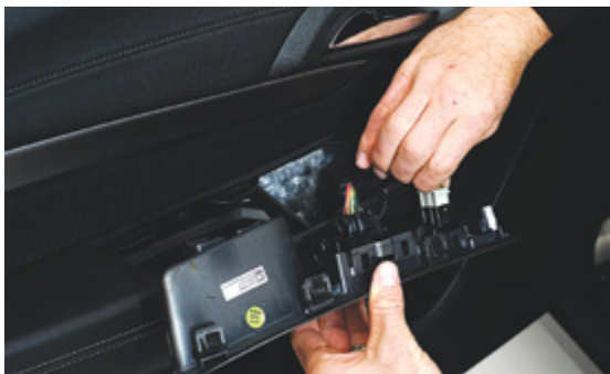
▲ Figure 14. Disconnecting the wiring harness
