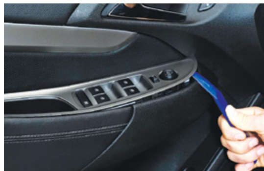
▲ Figure 13. Removing the window control panel from the door panel
