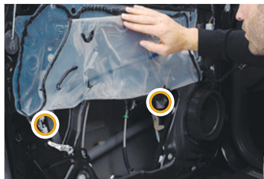
▲ Figure 21. Peeling back moisture barrier
