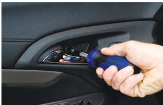
▲ Figure 10. Removing the 10 mm bolt from the interior door handle
