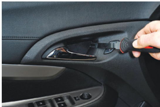
▲ Figure 9. Removing the trim cover behind the door handle
