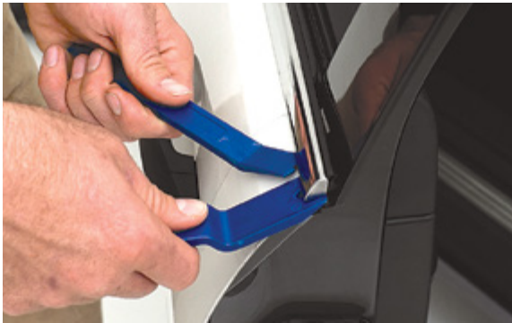
▲ Figure 23. Using the door pry tools to carefully release inner snap
