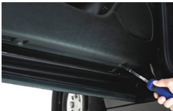
▲ Figure 8. Removing the two Phillips screws at the bottom of the interior door panel
