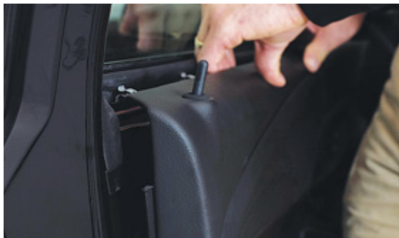
▲ Figure 18. Lifting the door panel over the lock pin
