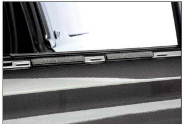
▲ Figure 15. Proper placement of Door Panel Grips
