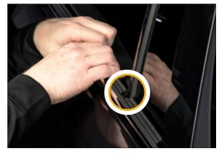
▲ Figure 16. Proper weatherstrip alignment
