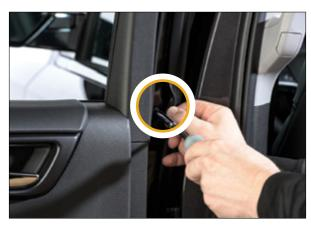
Figure 8. Exposing the front Torx screw
