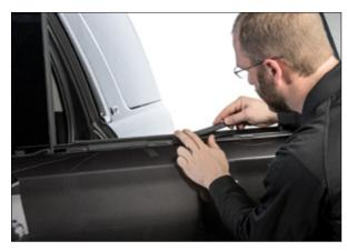
▲ Figure 14. Securing Door Panel Grips
