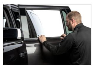
Figure 9. Removing the weatherstrip
