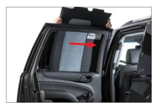
▲ Figure 11. Pushing panel forward while inserting panel
