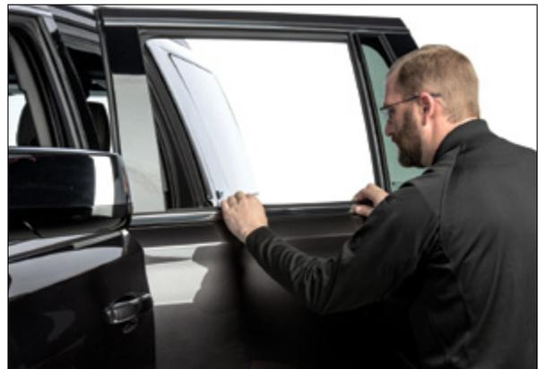
▲ Figure 9. Removing the weatherstrip
