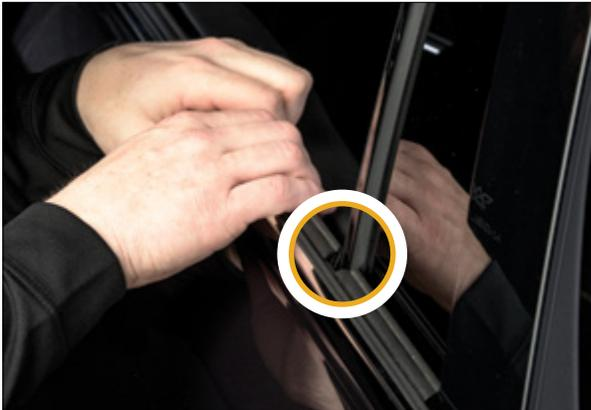
▲ Figure 16. Proper weatherstrip alignment
