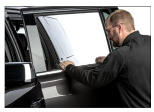
Figure 17. Pressing down to fully seat the weatherstrip
