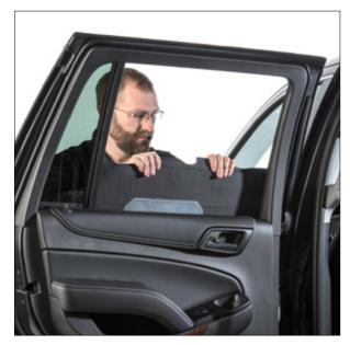
▲ Figure 12. Sliding panel down into the door
