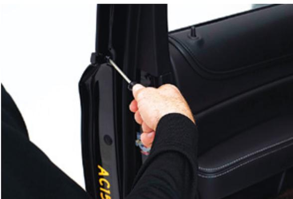
▲ Figure 17. Replacing outer window weatherstrip screw
