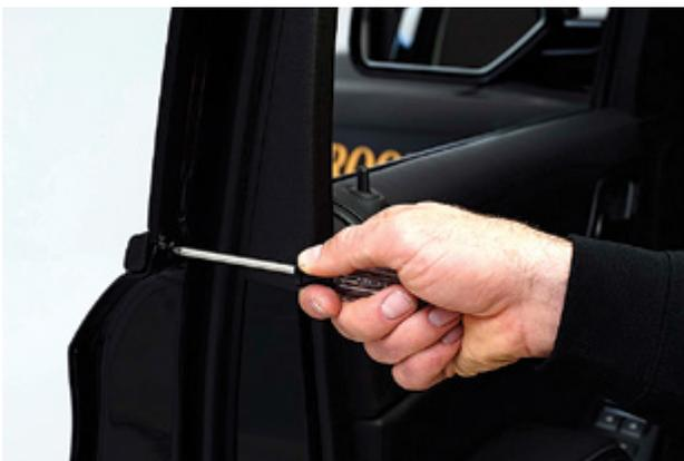
▲ Figure 8. Removing outer window weatherstrip screw
