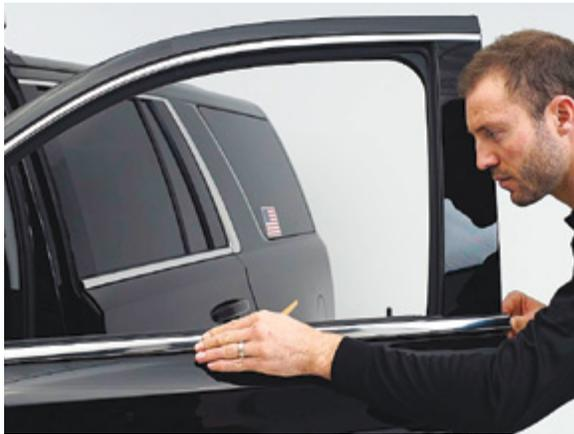
▲ Figure 16. Reinstalling outer window weatherstrip
