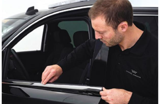
▲ Figure 9. Removing outer window weatherstrip
