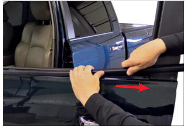
▲ Figure 8. Sliding back the outer window weatherstrip
