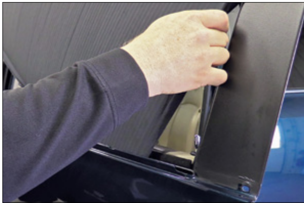
▲ Figure 10. Inserting panel between window glass and outer door skin
