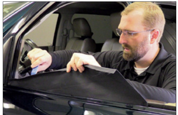
▲ Figure 12. Sliding panel toward front of door frame
