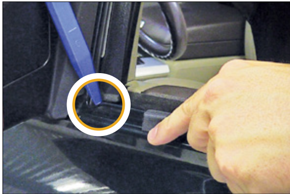
▲ Figure 13. Nylon fold is properly positioned on downward curve of the door seam
