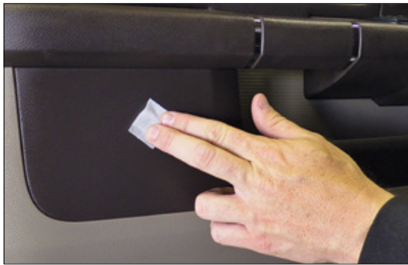
▲ Figure 17. Cleaning location with alcohol wipe
