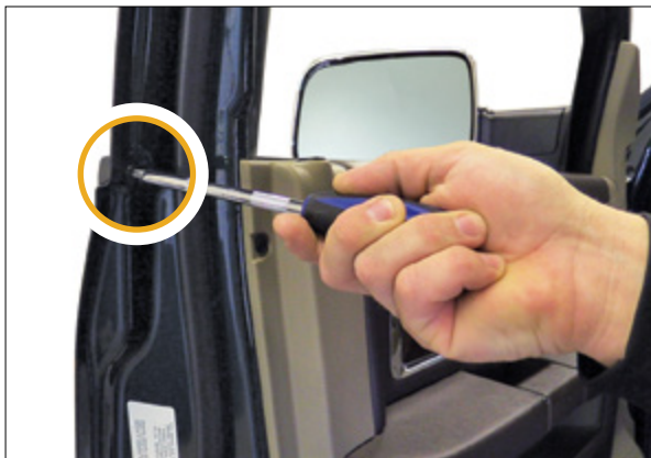
▲ Figure 7. Removing outer window weatherstrip Phillips-Head screw
