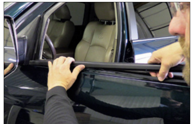
▲ Figure 15. Seating weatherstrip along window frame
