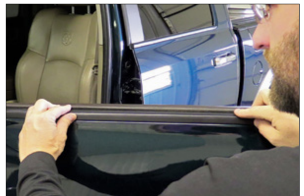
▲ Figure 16. Properly seated window weatherstrip
