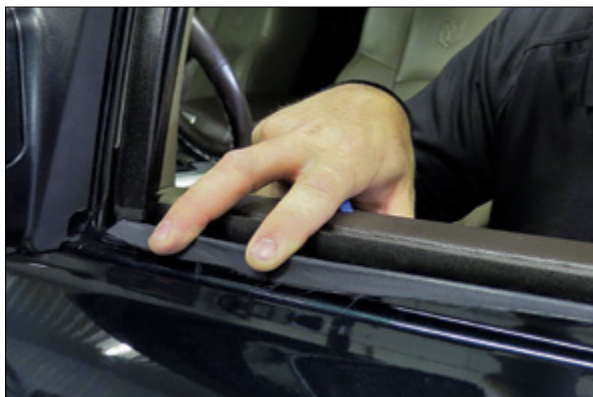
▲ Figure 14. Proper location of nylon fold
