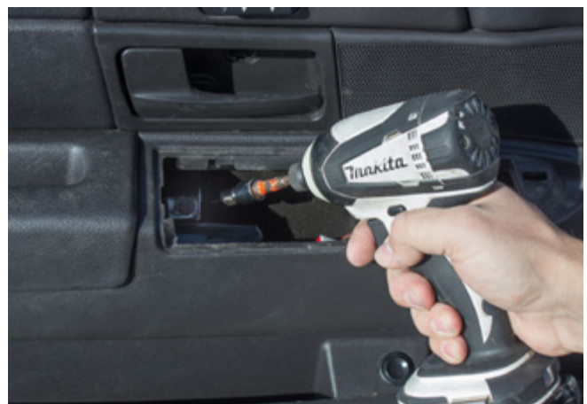
▲ Figure 12. Door control panel screw location
