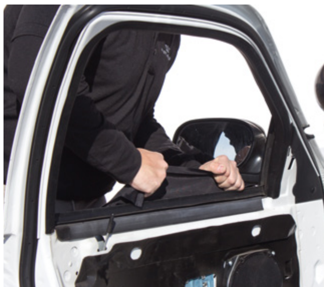
▲ Figure 20. Gripping ballistic door panel's top-edge nylon folds
