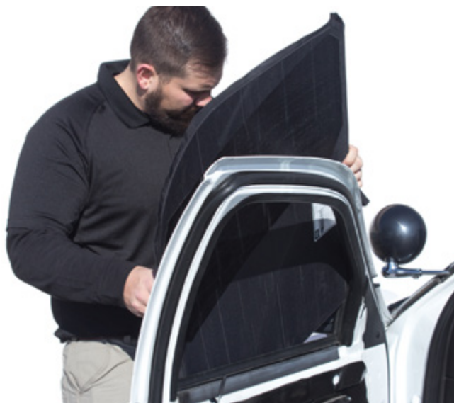
▲ Figure 19. Inserting the panel into the door
