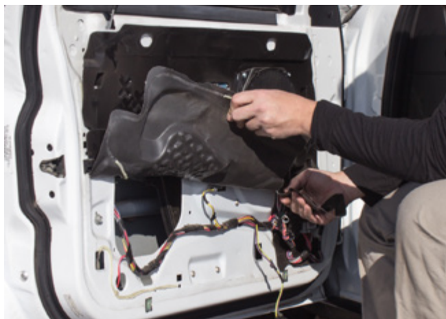
▲ Figure 15. Peeling back the moisture barrier to expose the window regulator
