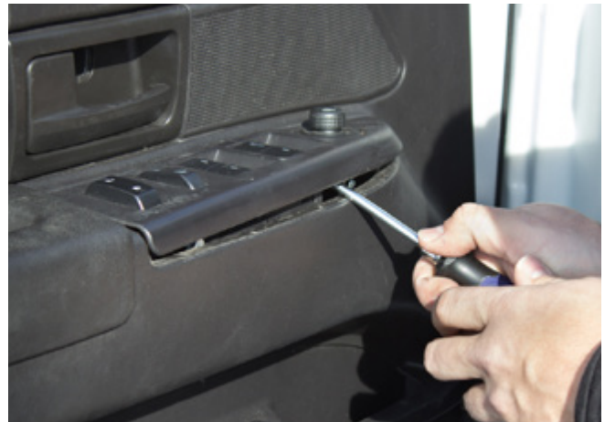
▲ Figure 11. Prying open door control panel
