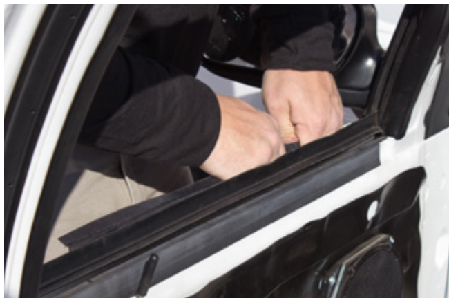
▲ Figure 21. Reaching into to door to feel the ballistic package, making sure it is below the internal sheet metal
