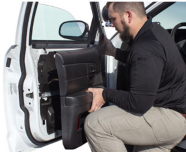
▲ Figure 13. Prying open the vehicle interior door trim panel
