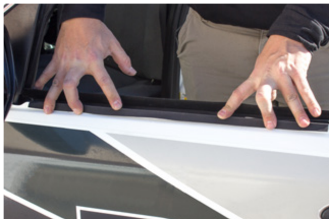
▲ Figure 22. Proper alignment of nylon fold with window frame
