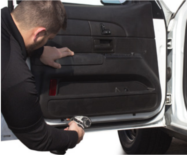
▲ Figure 9. Removing 7 mm panel mounting bolts
