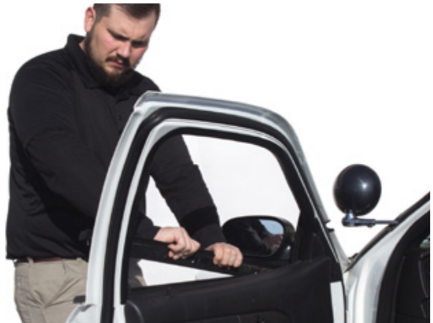
▲ Figure 8. Removing the window trim
