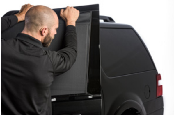
▲ Figure 10. Holding Ballistic Door Panel against window glass while leaning back
