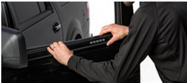
▲ Figure 15. Positioning the weatherstrip onto the window frame and under side mirror
