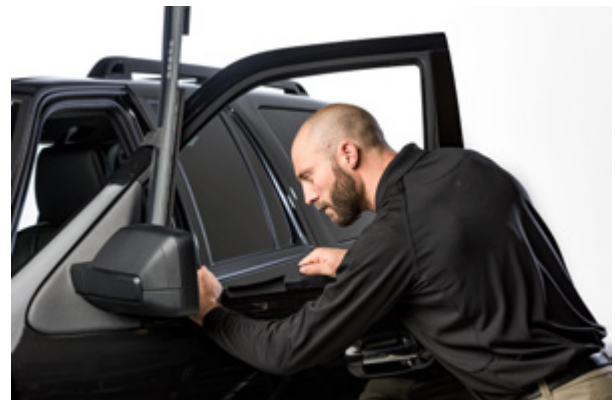
▲ Figure 12. Gripping and sliding the Ballistic Door Panel forward into place
