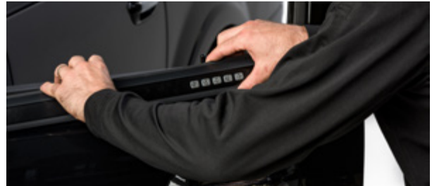
▲ Figure 16. Pressing the weatherstrip into the window frame
