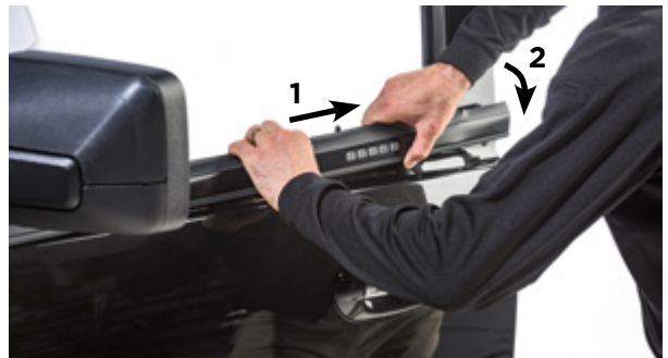
▲ Figure 8. Removing the outer window weatherstrip
