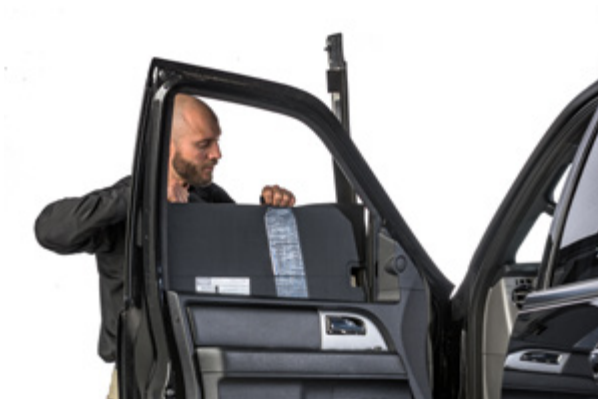
▲ Figure 11. Sliding Ballistic Door Panel into the door
