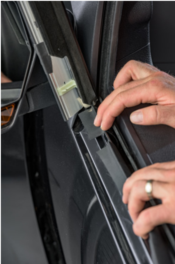
▲ Figure 13. Proper alignment of nylon fold with edge of window frame
