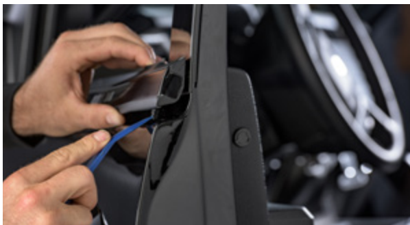
▲ Figure 7. Releasing inner snap on outer window weatherstrip
