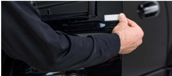
▲ Figure 14. Adhering the adhesive strip to the damaged snap
