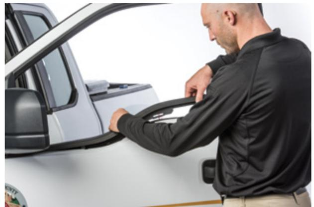
▲ Figure 8. Removing the outer window weatherstrip
