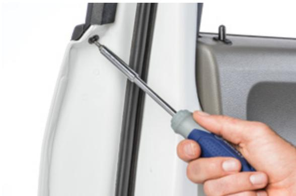
▲ Figure 14. Replacing outer window weatherstrip screw
