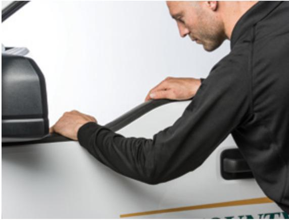
▲ Figure 13. Reinstalling outer window weatherstrip
