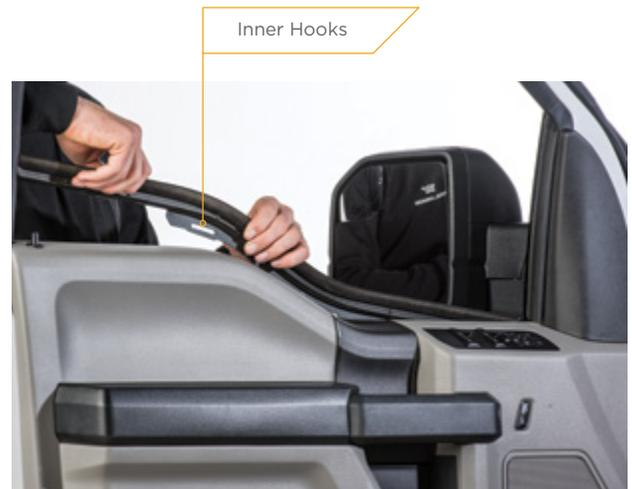
▲ Figure 7. Releasing the inner hooks
