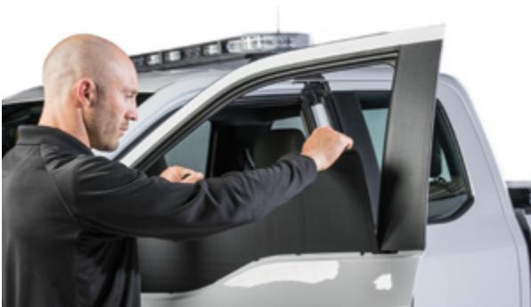
▲ Figure 10. Holding Ballistic Door Panel against window glass while leaning back
