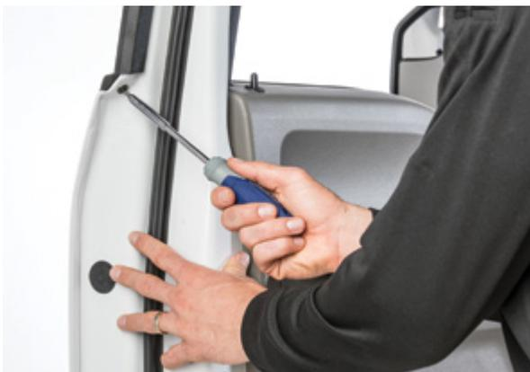
▲ Figure 6. Removing outer window weatherstrip screw
