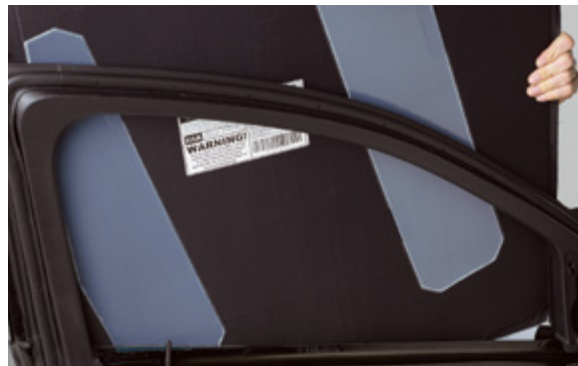
▲ Figure 29. Proper placement of the ballistic panel before insertion
