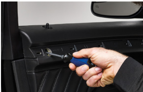
▲ Figure 12. Removing the 8 mm bolt behind the trim bar
