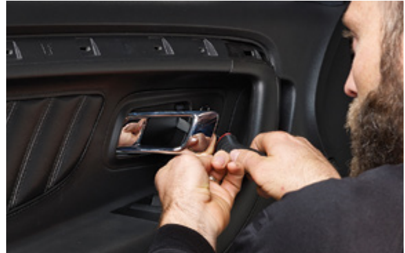
▲ Figure 8. Removing the trim cover behind the door handle
