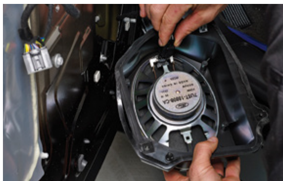
▲ Figure 24. Disconnecting the speaker wiring harness
