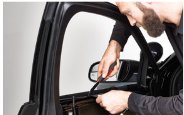
▲ Figure 28. Using the pry tools to push the ballistic panel down and under the outside sheet metal lip
