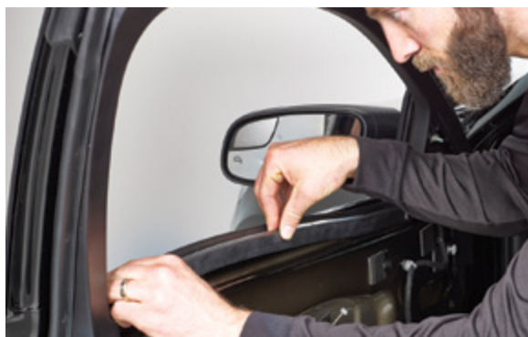
▲ Figure 33: Replacing the interior weatherstrip
