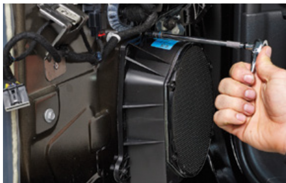
▲ Figure 22. Removing the speaker screws
