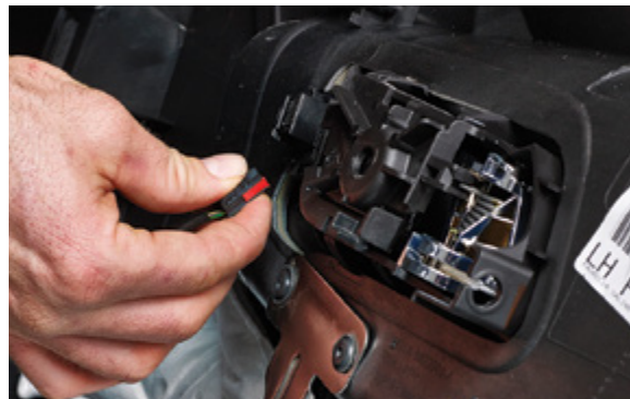
▲ Figure 20. Disconnecting the wiring harness
