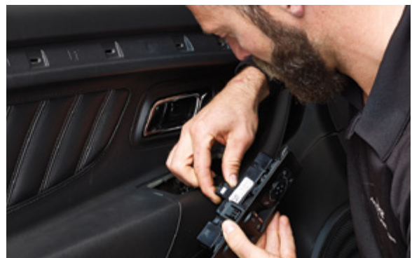
▲ Figure 10. Disconnecting the wiring harness
