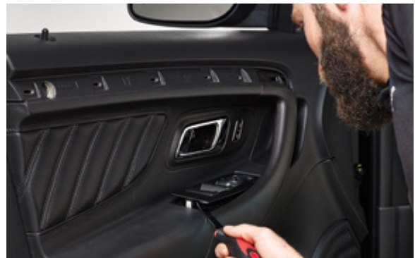
▲ Figure 9. Removing the window control panel
