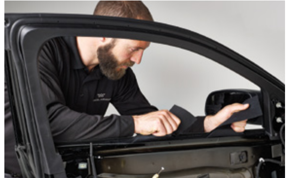
▲ Figure 27. Gripping ballistic door panel's top-edge nylon folds and sliding the panel forward
