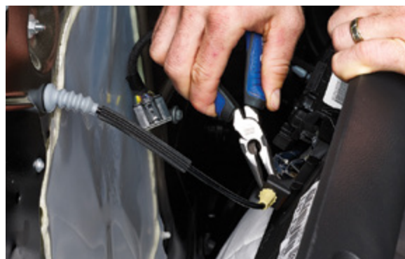
▲ Figure 21. Disconnecting the door latch cable
