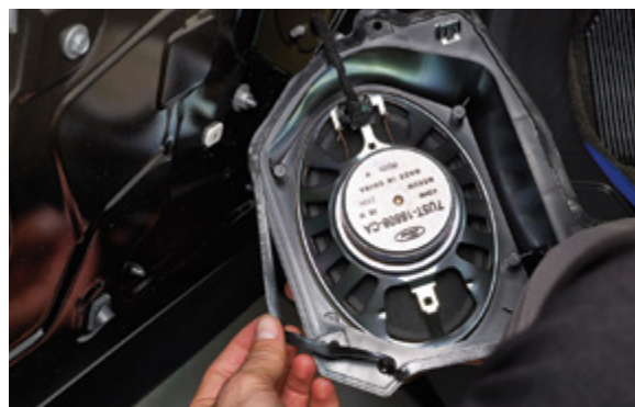
▲ Figure 32. Re-installing the speaker gasket
