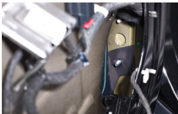
▲ Figure 30. Nylon tab placed over the replacement bolt
