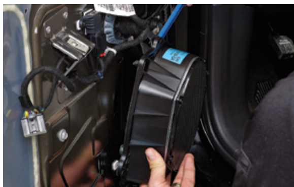
▲ Figure 23. Prying the speaker from the door panel
