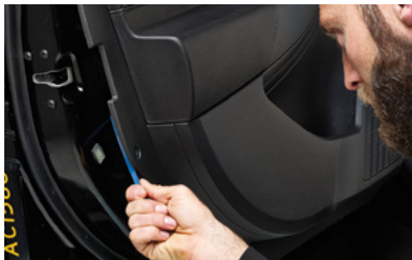
▲ Figure 17. Prying the door panel away from the door
