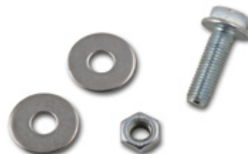
▲ Figure 6. One M8x1.25x35mm hex head bolt, two M8 fender washers and one M8x1.25 lock nut
