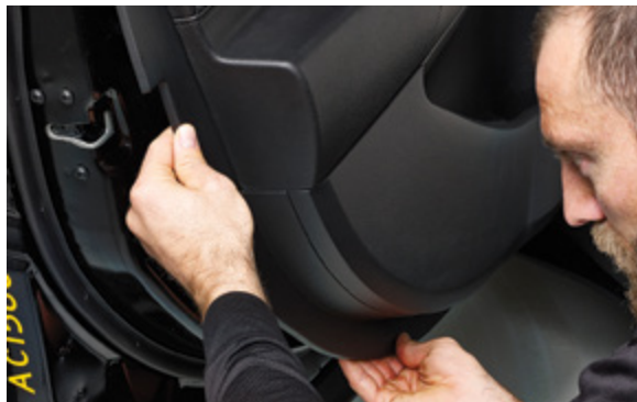
▲ Figure 18. Working around the door panel to release snaps
