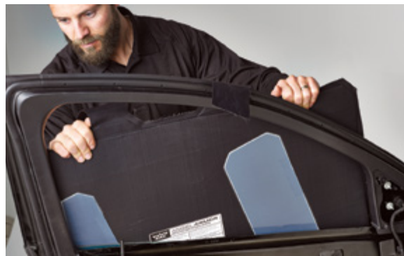
▲ Figure 30. Sliding the panel down into the door
