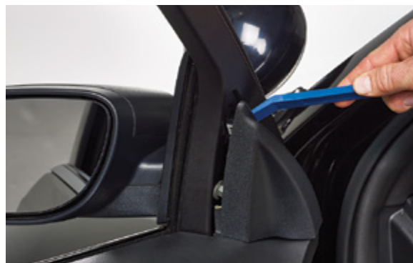
▲ Figure 16. Removing the side mirror cover
