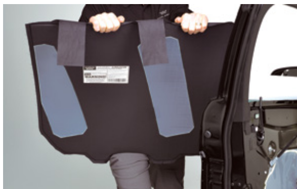
▲ Figure 28. Bending the ballistic panel to create a slight curve
