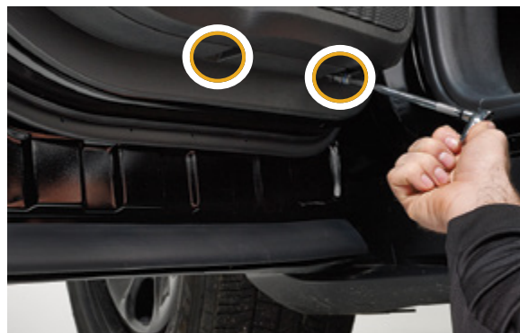
▲ Figure 15. Removing the two 7 mm bolts from behind the bottom of the door panel.
