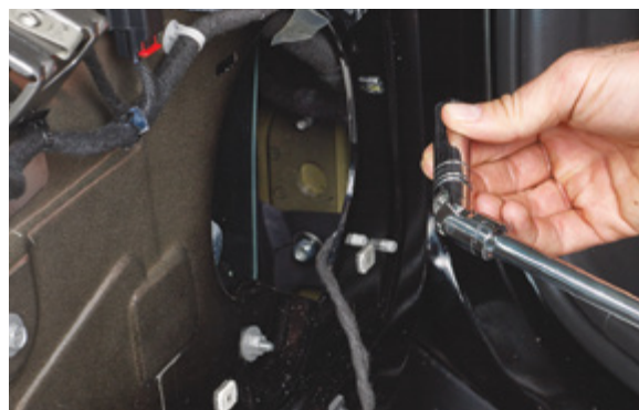
▲ Figure 31. Tightening the lock nut for proper installation
