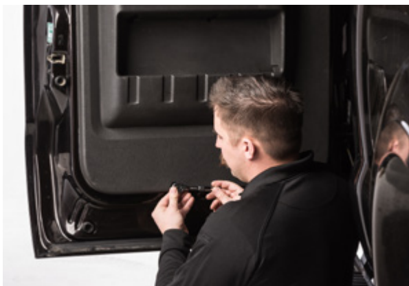
▲ Figure 9. Removing door compartment screws
