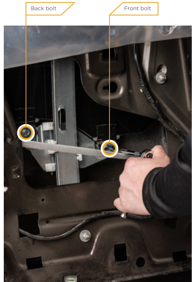
▲ Figure 16. Replacing the window bolts
