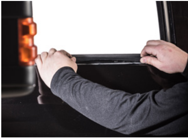
▲ Figure 22. Positioning the nylon folds over the window frame
