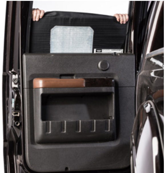
▲ Figure 21. Inserting the Avail Ballistic Door Panel into the door
