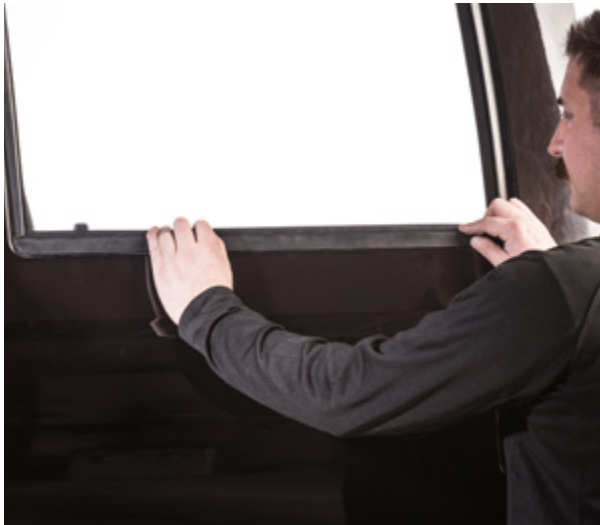
▲ Figure 19. Removing the window weatherstrip
