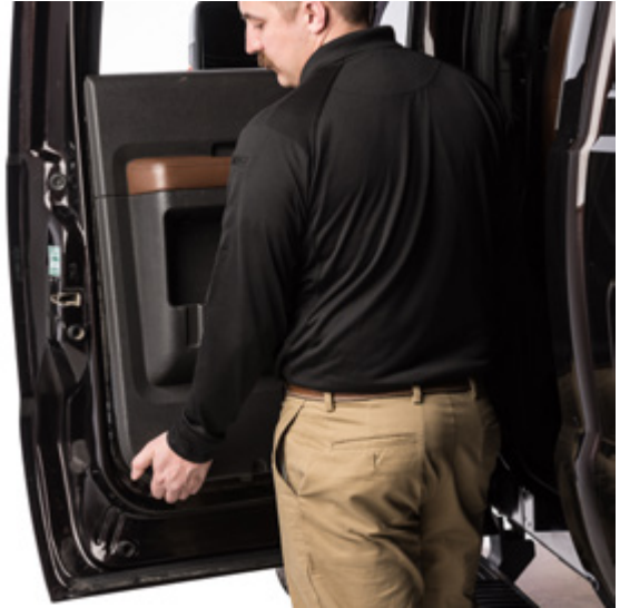
▲ Figure 13. Pulling the door panel up and away from the door
