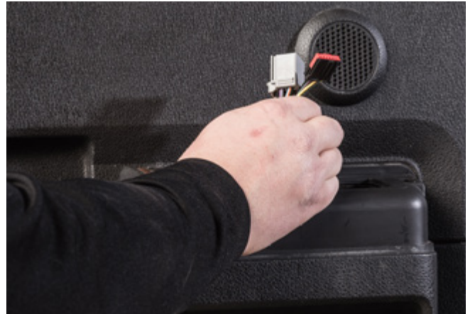
▲ Figure 18. Ensuring the wiring harnesses are visible
