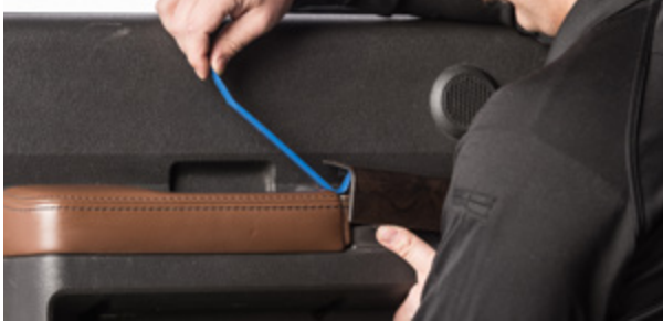
▲ Figure 11. Removing the window control panel
