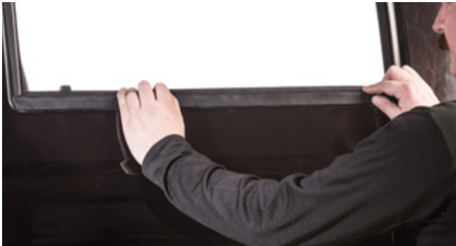
▲ Figure 23. Pressing down the window weatherstrip
