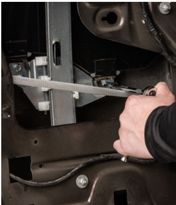
▲ Figure 15. Removing the regulator bolts
