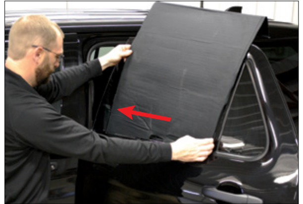
▲ Figure 11. Pushing panel forward toward front window frame
