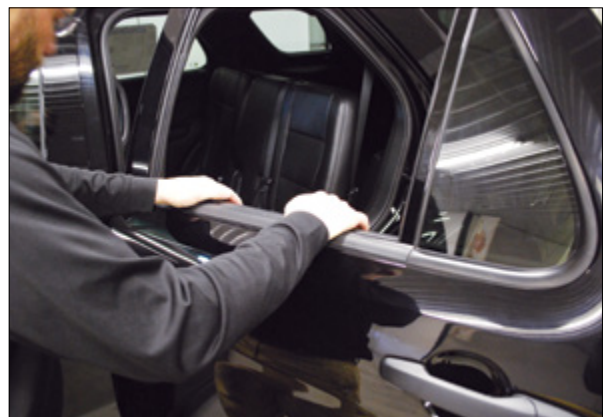
▲ Figure 15. Securing the weatherstrip
