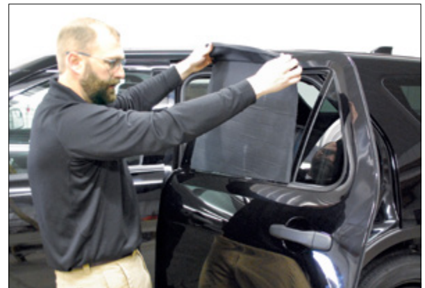
▲ Figure 12. Sliding panel down into the door
