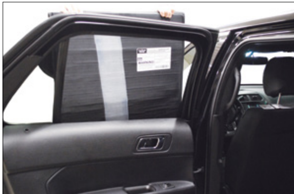
▲ Figure 10. Anti-abrasion panel facing interior of vehicle
