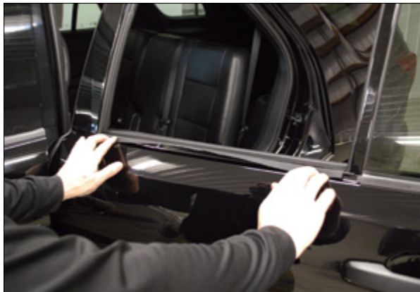
▲ Figure 13. Proper location of nylon fold
