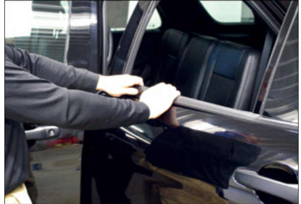
▲ Figure 7. Removing the weatherstrip
