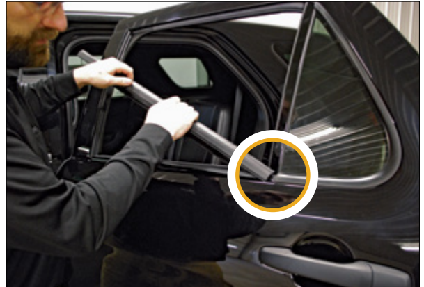
▲ Figure 14. Replacing the weatherstrip
