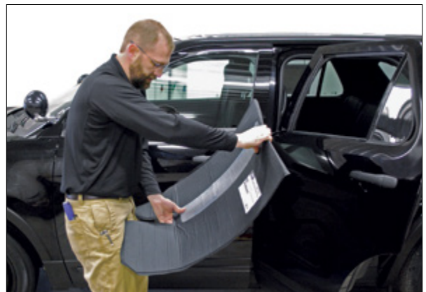
▲ Figure 8. Bending the Ballistic Door Panel to create a slight curve
