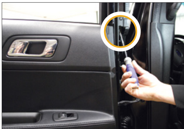
▲ Figure 6. Removing the front Torx screw
