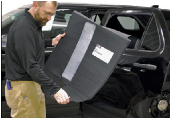
▲ Figure 9. Bending the bottom-right tab of Ballistic Door Panel to create a slight curve
