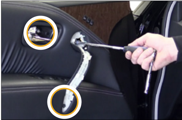
▲ Figure 11. Removing 10mm bolts
