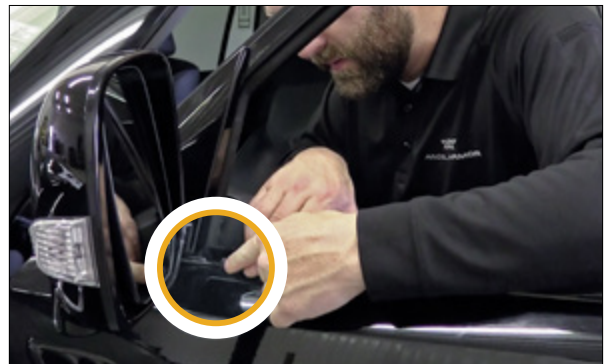
▲ Figure 26. Ensuring the panel is in correct location
