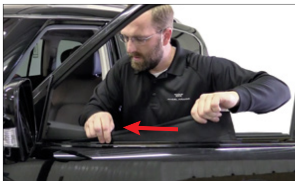
▲ Figure 24. Sliding panel forward while pushing down
