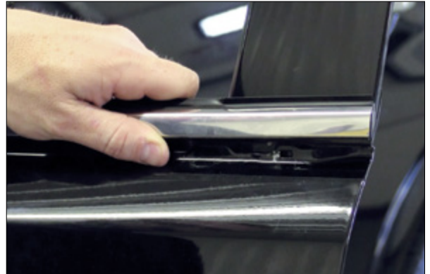
▲ Figure 18. Releasing first weatherstrip retaining clip
