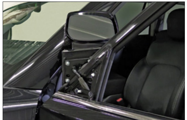
▲ Figure 14. Propping side-view mirror away from weatherstrip
