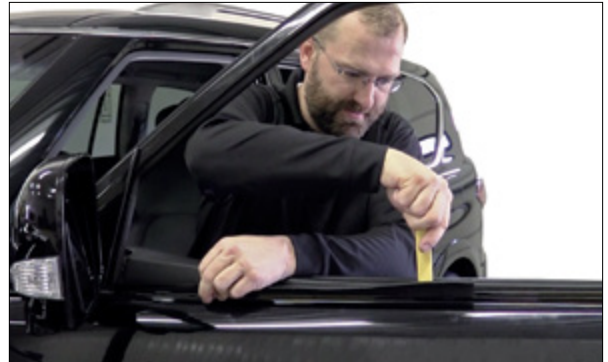
▲ Figure 25. Pushing down panel using plastic door pry tool
