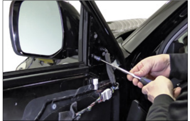
▲ Figure 13. Removing 10mm bolts from side-view mirror panel
