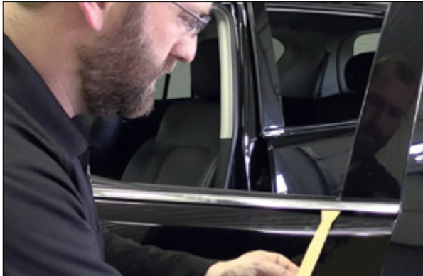
▲ Figure 16. Creating gap between weatherstrip and window frame
