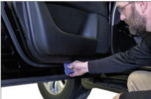
▲ Figure 12. Prying door panel from door
