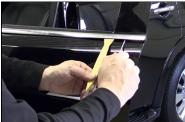
▲ Figure 17. Inserting pick tool under lifted weatherstrip
