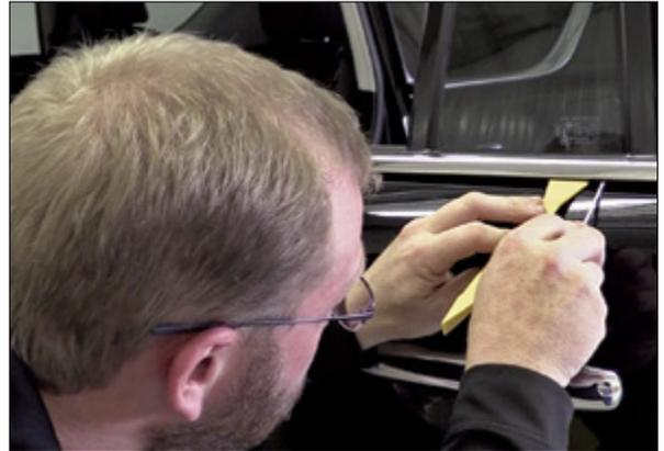
▲ Figure 7. Inserting pick tool under lifted weatherstrip
