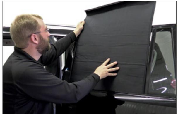
▲ Figure 10. Inserting panel into door
