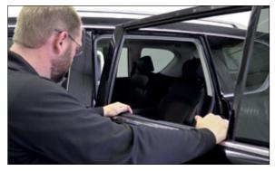
Figure 14. Pressing down to fully seat the weatherstrip
