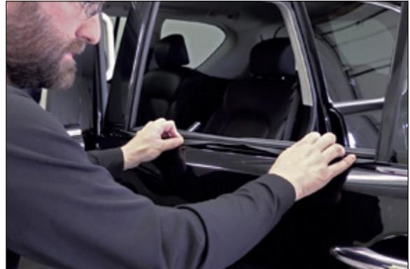
▲ Figure 12. Nylon sitting flush where weatherstrip is installed
