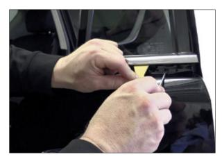
▲ Figure 8. Releasing first weatherstrip retaining clip
