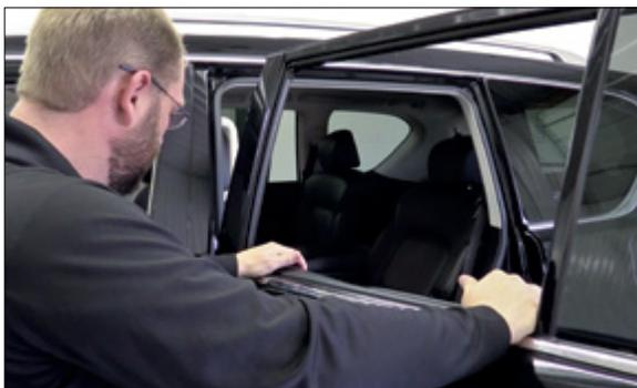
▲ Figure 14. Pressing down to fully seat the weatherstrip
