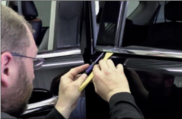
▲ Figure 9. Releasing second weatherstrip retaining clip
