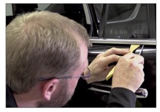
▲ Figure 7. Inserting pick tool under lifted weatherstrip
