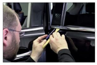
Figure 9. Releasing second weatherstrip retaining clip
