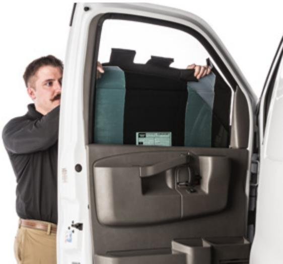
▲ Figure 9. Inserting ballistic panel into door with anti-abrasion panels facing vehicle interior
