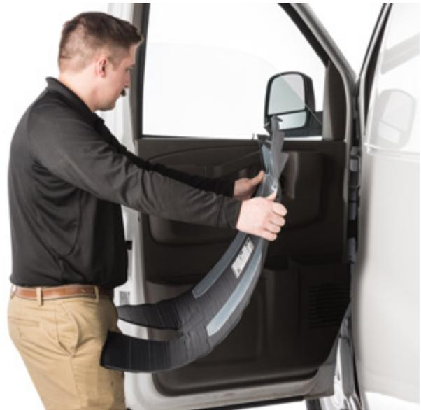
▲ Figure 7. Bending ballistic panel to match curve of the door
