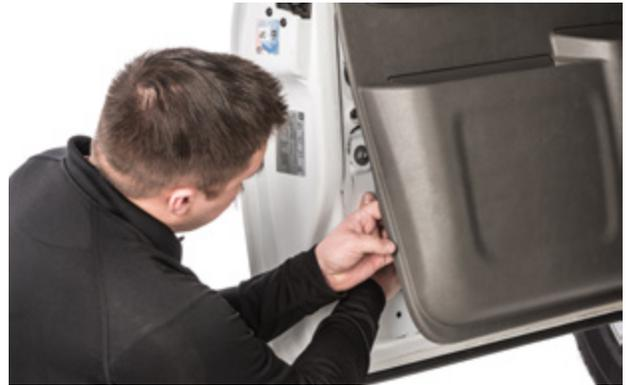
▲ Figure 10. Reaching in through holes to adjust internal wire
