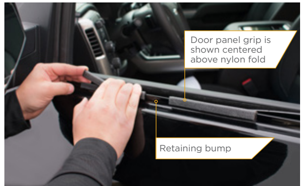
▲ Figure 14. Proper alignment of door panel grips.
