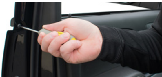
▲ Figure 17. Replacing outer window weatherstrip screw
