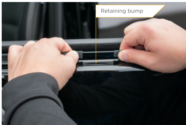
▲ Figure 13. Proper alignment of nylon fold with window frame.
