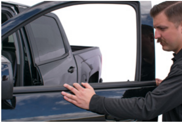
▲ Figure 16. Reinstalling outer window weatherstrip
