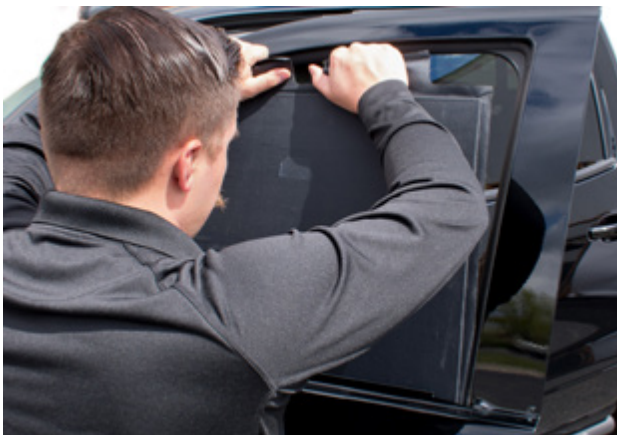
▲ Figure 11. Holding ballistic door panel against window glass while leaning back
