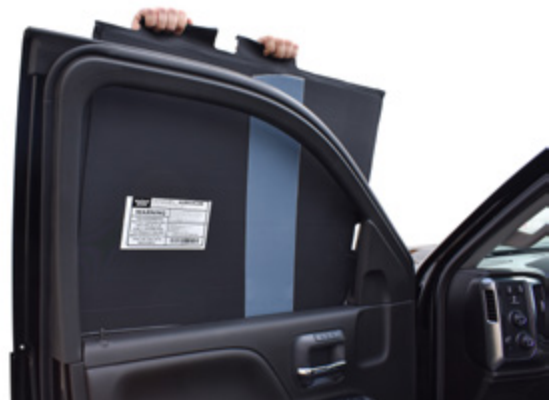
▲ Figure 10. Inserting ballistic panel into door with anti-abrasion panels facing vehicle interior
