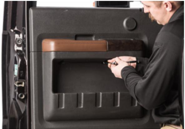
▲ Figure 10. Removing the bolt cover
