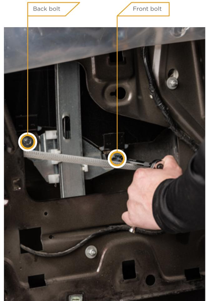
▲ Figure 16. Replacing the window bolts
