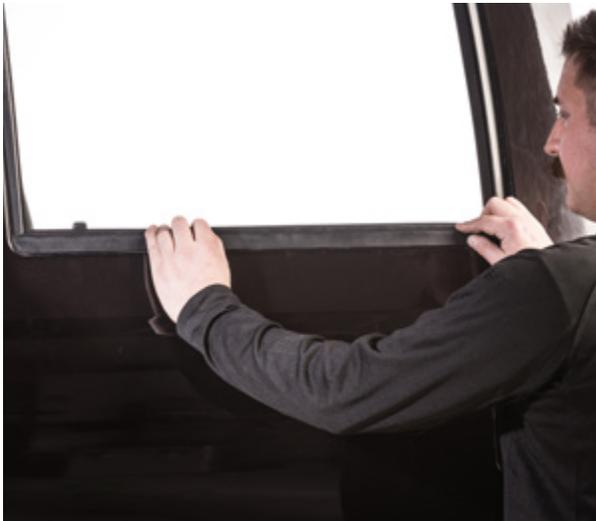
▲ Figure 19. Removing the window weatherstrip
