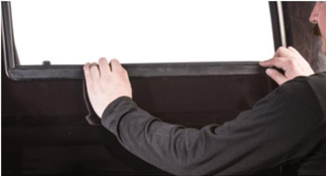
▲ Figure 23. Pressing down the window weatherstrip
