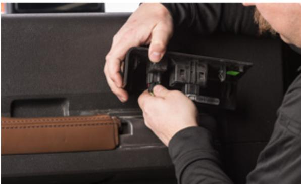
▲ Figure 12. Disconnecting the wiring harnesses
