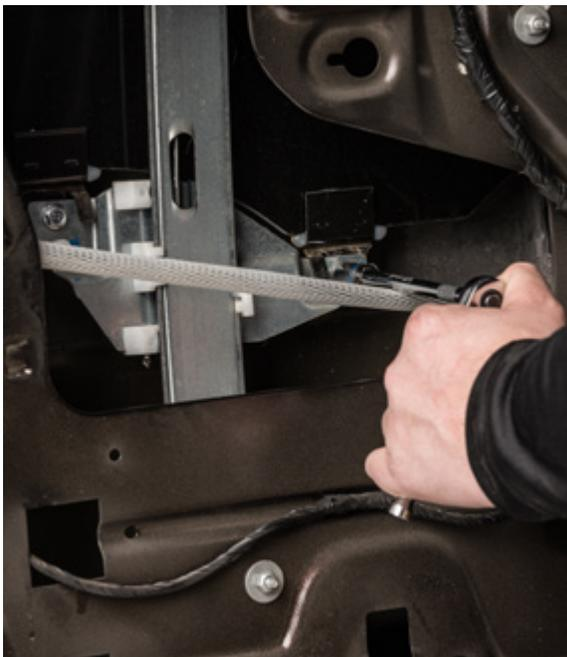
▲ Figure 15. Removing the regulator bolts
