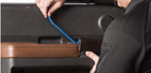
▲ Figure 11. Removing the window control panel
