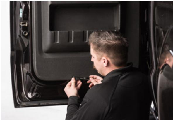
▲ Figure 9. Removing door compartment screws
