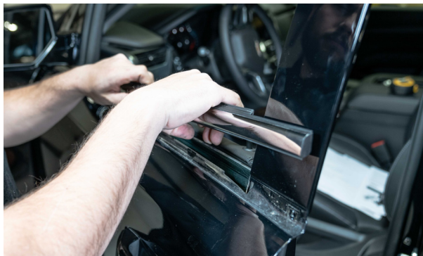
▲ Figure 24. Removing the outer window weatherstrip.
