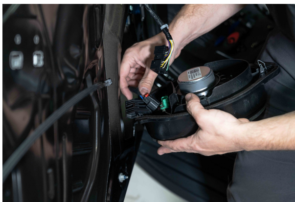
▲ Figure 31. Disconnecting the speaker harness.
