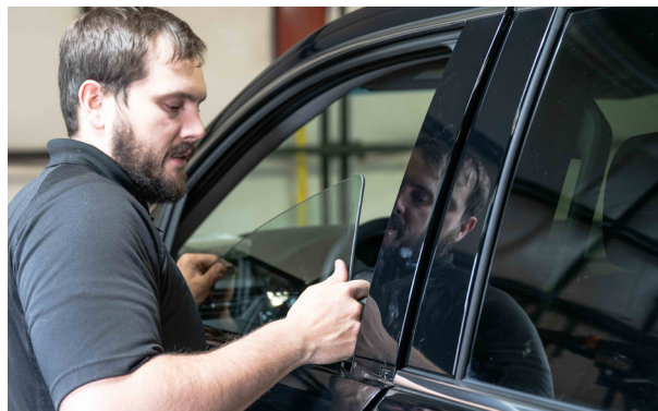
▲ Figure 39. Removing the window glass.
