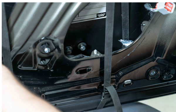
▲ Figure 57. The front, top of the crash bar bracket loosely installed .
