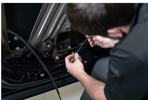
▲ Figure 73. Installing the lower mounting bracket.
