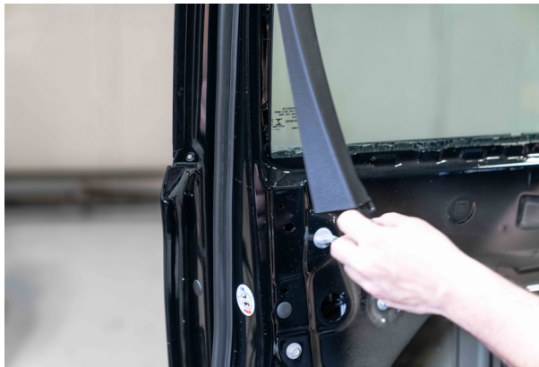
▲ Figure 35. Removing the window trim.
