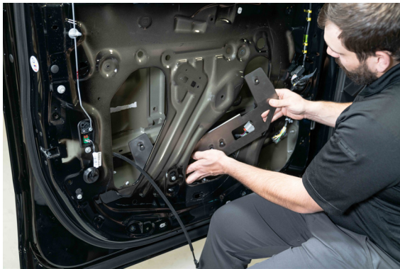
▲ Figure 50. Inserting the Crash Bar Mounting Bracket through the door opening.
