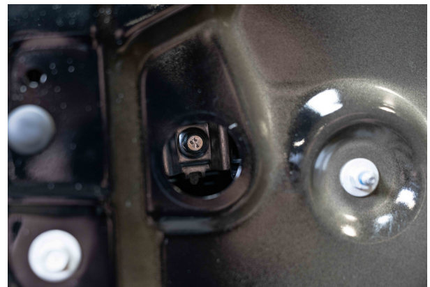
▲ Figure 37. Window regulator bolt head pictured through the inner door skin.
