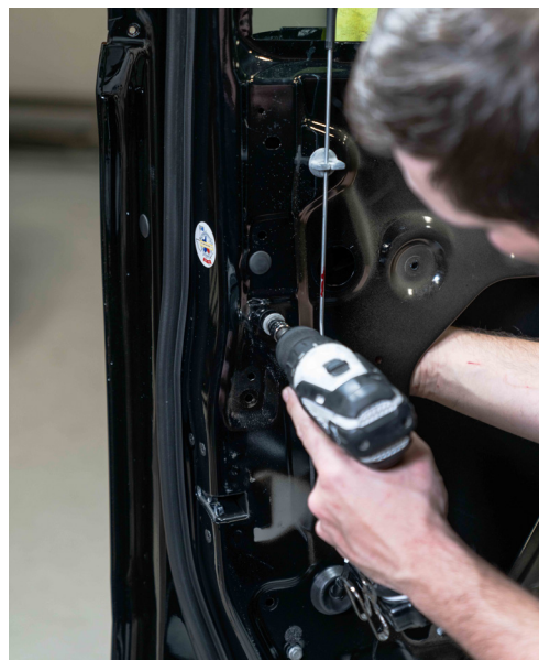
▲ Figure 75. Remove the upper window track bolt.
