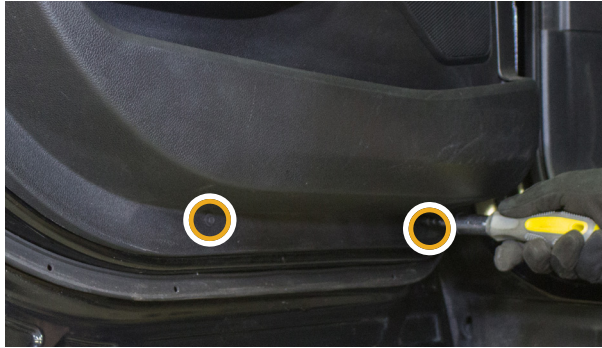
▲ Figure 27. Removing the door panel bolts.
