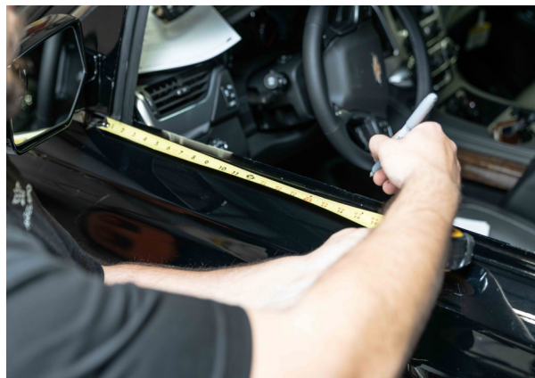
▲ Figure 45. Marking Bracket locations.
