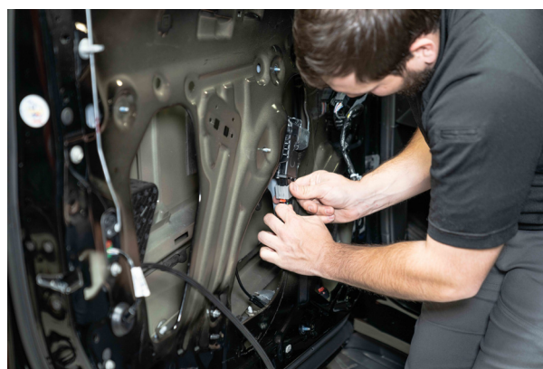
▲ Figure 40. Disconnecting the window regulator wiring harness.
