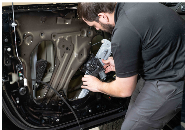
▲ Figure 42. Removing the window regulator.
