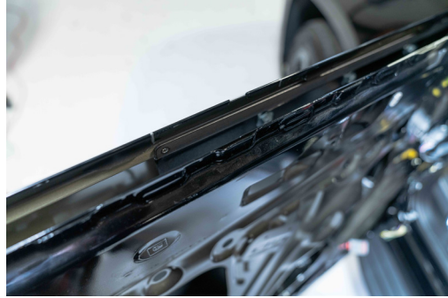
▲ Figure 66. Support Bracket aligned and installed.
