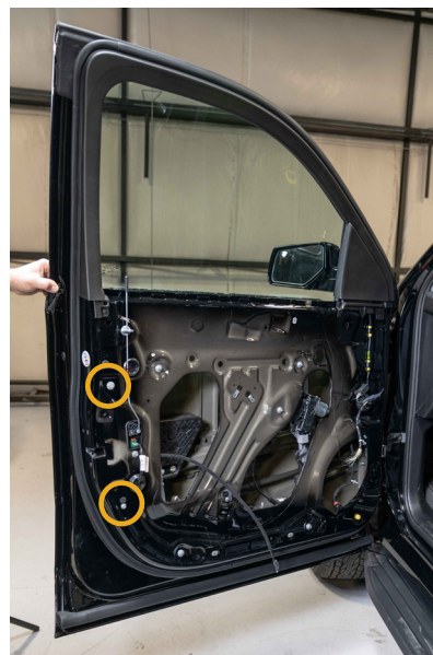
▲ Figure 74. Mounting locations for the rear window track.
