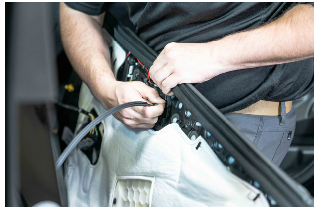
▲ Figure 30. Removing the door latch cable.
