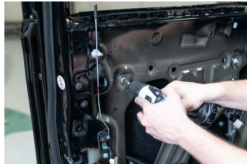
▲ Figure 72. Tightening the regulator mounting bolt.
