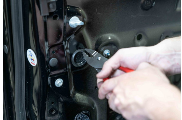
▲ Figure 36. Removing the rear regulator bolt cover.
