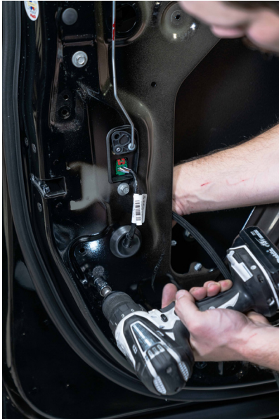
▲ Figure 76. Loosening the rear window track.
