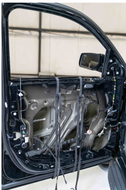
▲ Figure 53. Looping the installation straps around the door.
