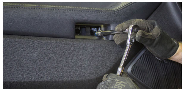
▲ Figure 26. Removing the armrest pocket bolts.
