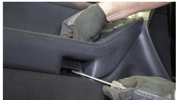
▲ Figure 25. Removing the armrest pocket trim cover.
