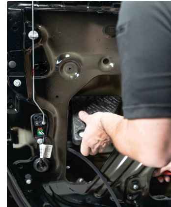
▲ Figure 48. Prying out the foam block.
