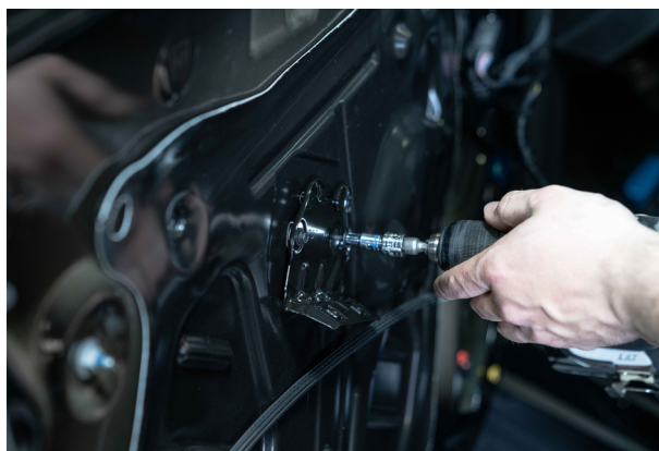
▲ Figure 32. Removing the door handle bracket.
