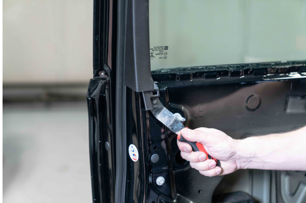
▲ Figure 34. Removing the rear clip of the window trim.
