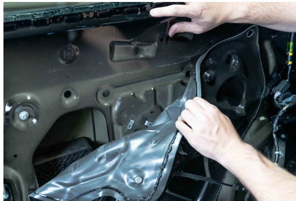
▲ Figure 33. Removing the weather seal.
