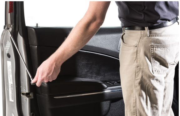
▲ Figure 30. Removing the back window weatherstrip screw.
