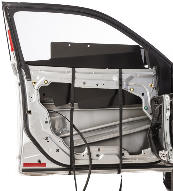
▲ Figure 49. Proper placement of the armor installed \frac{3}{4} of the way into the door.
