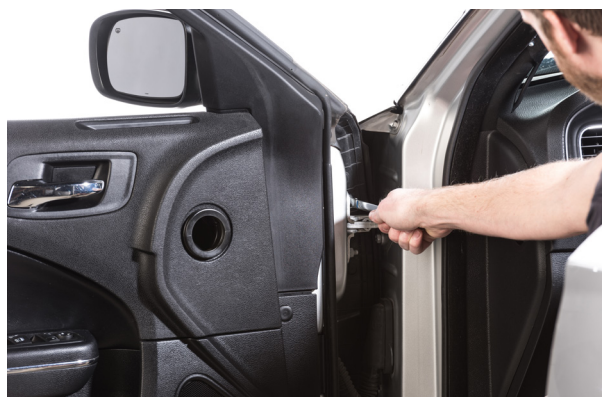
▲ Figure 20. Removing the upper door hinge bolt and nut.
