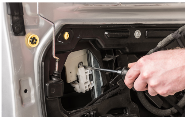
▲ Figure 42. Releasing the back window clip.
