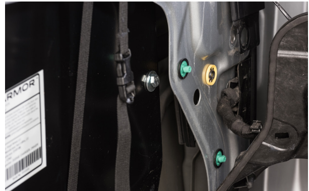
▲ Figure 50. The front, top crash bar bracket loosely installed.
