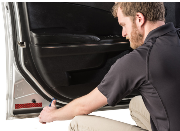
▲ Figure 37. Prying the door panel away from the door skin.
