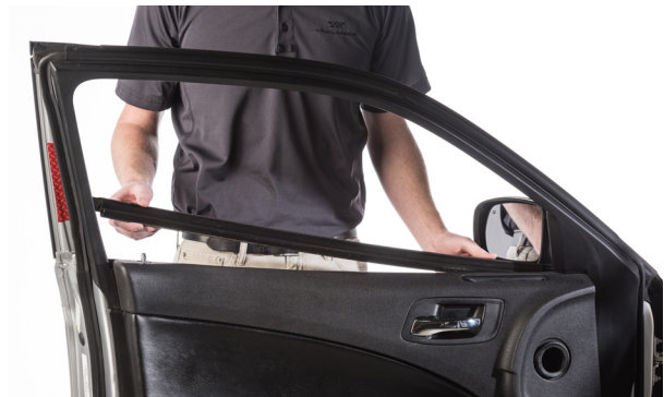
▲ Figure 31. Removing the outer window weatherstrip.
