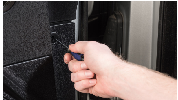
▲ Figure 35. Removing the fastener at the inner edge of the door panel.
