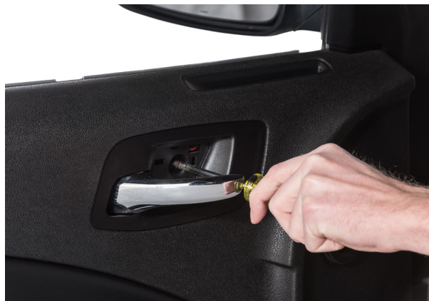
▲ Figure 33. Removing the interior door handle screw.
