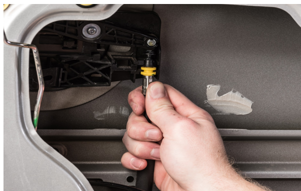
▲ Figure 44. Disconnecting the cable from the door handle mechanism.
