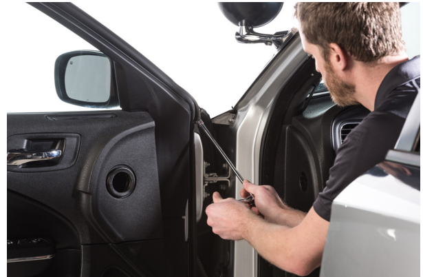
▲ Figure 29. Removing the front window weatherstrip screw.
