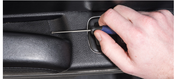
▲ Figure 34. Removing the armrest pocket trim cover.
