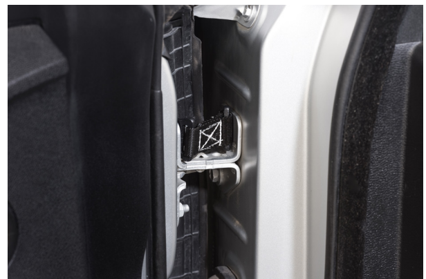
▲ Figure 28. Proper placement of the secured check strap.
