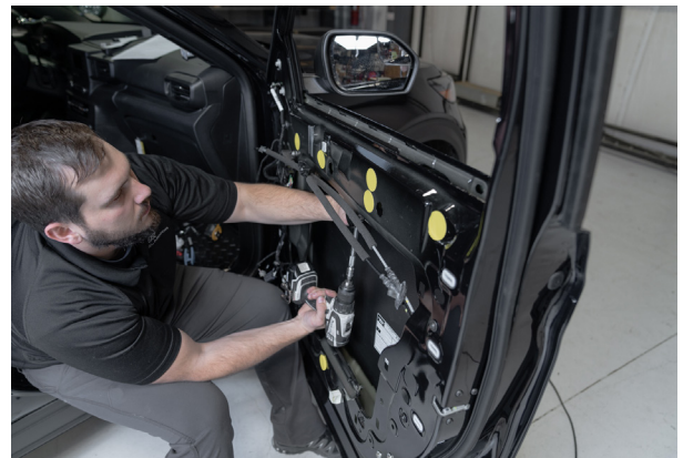
▲ Figure 61. Screwing the sheet metal screws into the upper door frame through the support and upper bracket.
