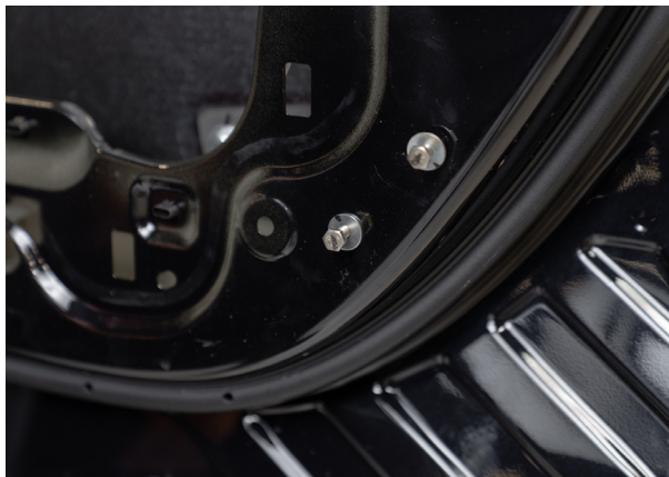
▲ Figure 56. Lower mounting bracket loosely installed.
