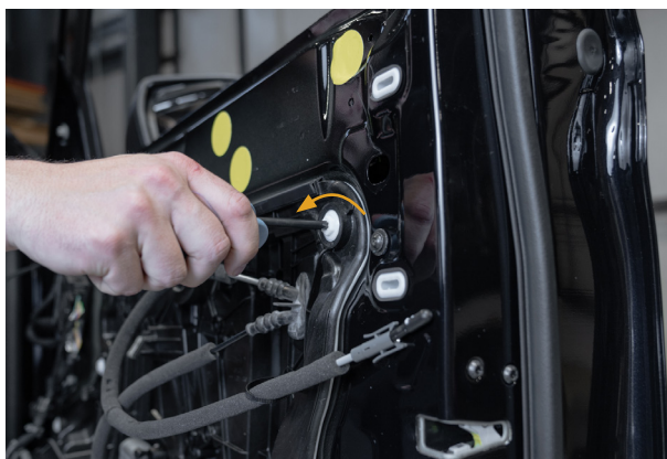
▲ Figure 35. Rotating Torx Clips.
