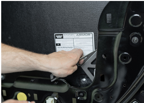
▲ Figure 55. Inserting Lower Mounting Bracket.
