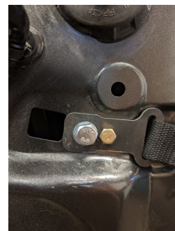
▲ Figure 45. Check strap mounting on the door.
