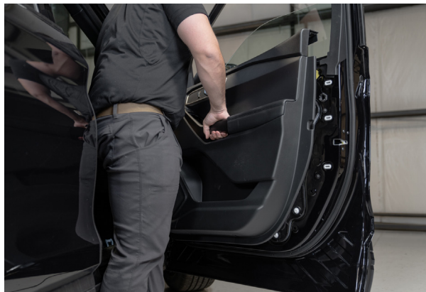
▲ Figure 28. Removing the door panel.
