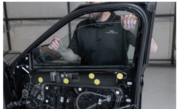
▲ Figure 33. Removing the window glass.
