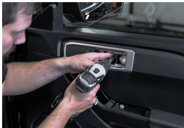
▲ Figure 23. Removing the interior door handle bolt.
