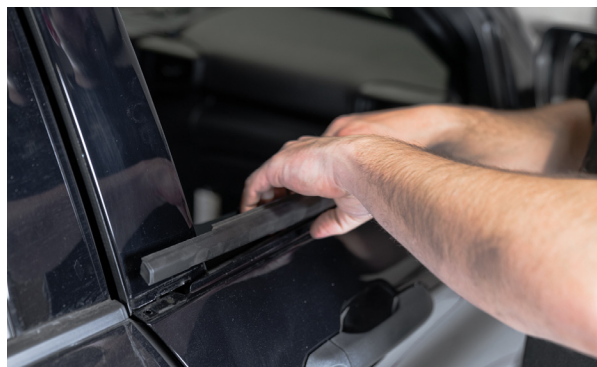
▲ Figure 21. Removing the outer window weatherstrip.
