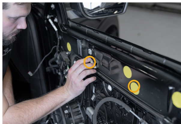
▲ Figure 36. Removing the adhesive patches.
