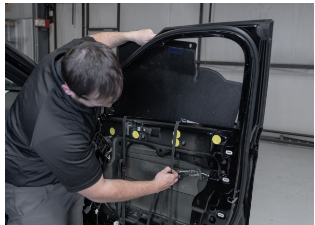
▲ Figure 52. Using the cradle created by the installation straps to lower the armor into the door.
