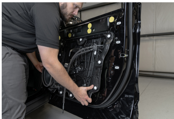
▲ Figure 38. Removing window regulator panel.
