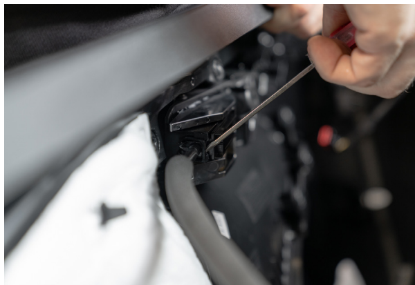
▲ Figure 29. Unclipping the door latches.
