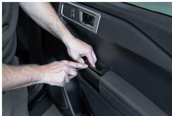
▲ Figure 24. Removing the interior door handle bolt.
