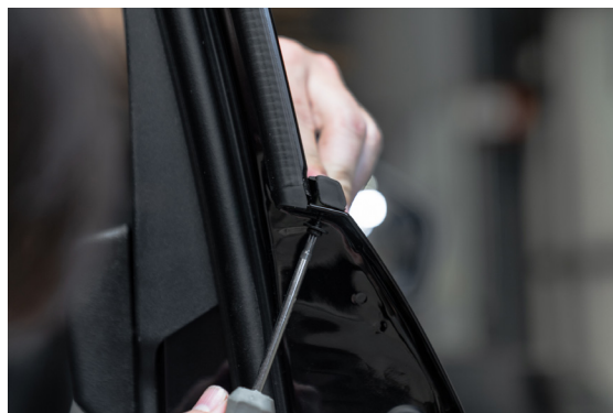
▲ Figure 20. Removing the back window weatherstrip screw.
