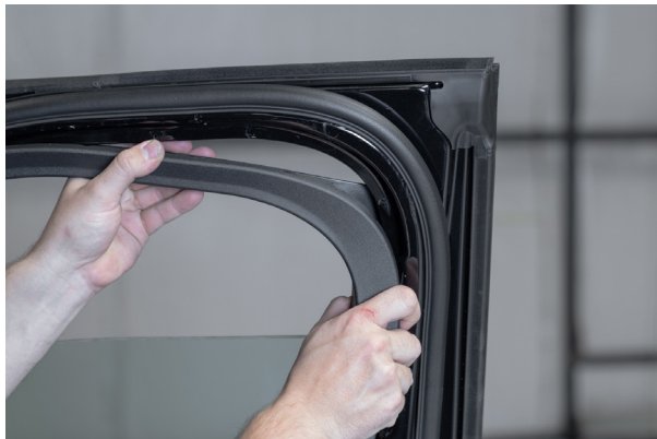
▲ Figure 43. Removing window trim.
