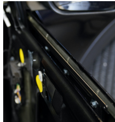
▲ Figure 58. The support bracket dry fitted into door.
