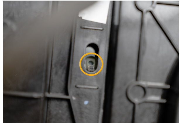
▲ Figure 32. Locating the window regulator clips.
