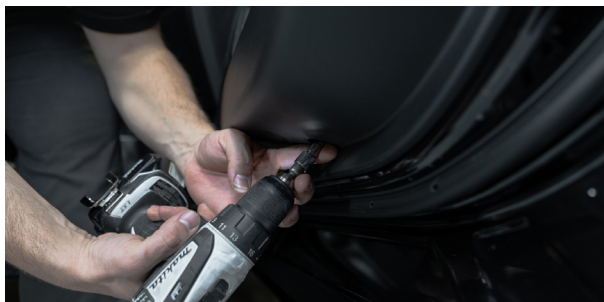
▲ Figure 26. Removing the lower panel bolts.
