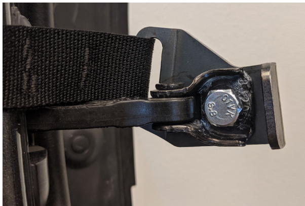
▲ Figure 46. Check strap orientation on A-pillar.
