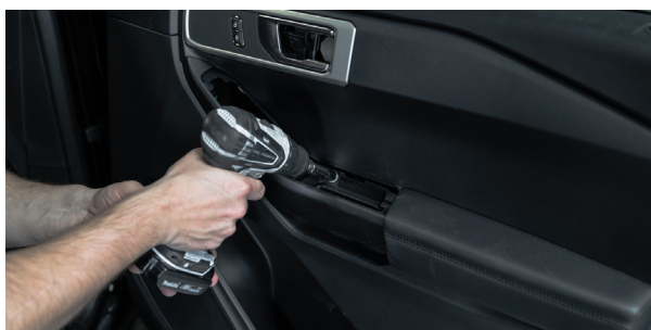
▲ Figure 25. Removing the armrest pocket bolts.
