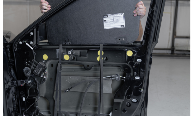
▲ Figure 51. Placing the armor into the door.
