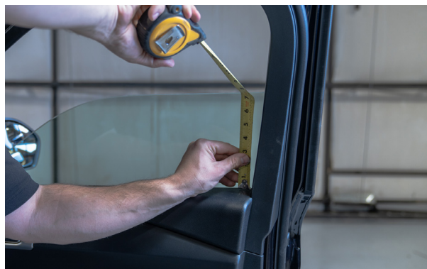
▲ Figure 31. Measuring the window height.
