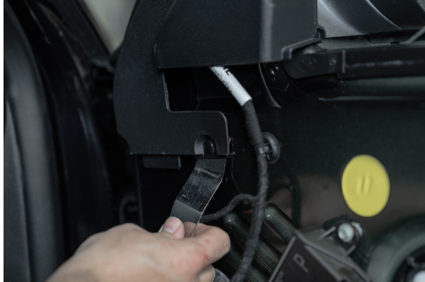
▲ Figure 42. Removing window trim from clips.
