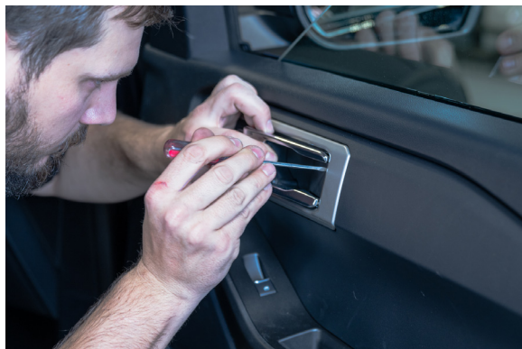
▲ Figure 22. Remove the interior door handle trim cover.
