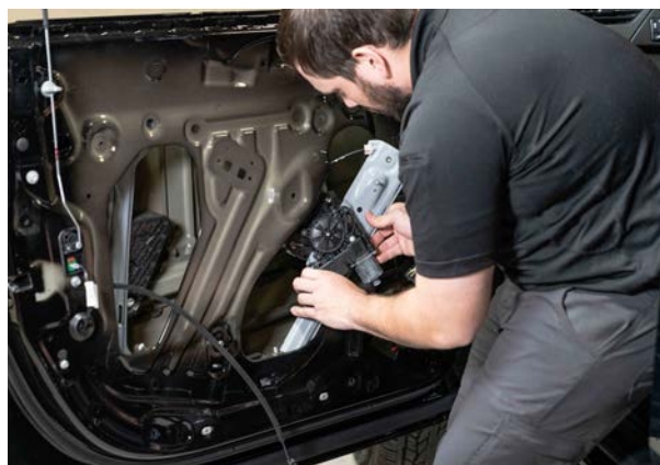
▲ Figure 39. Removing the window regulator
