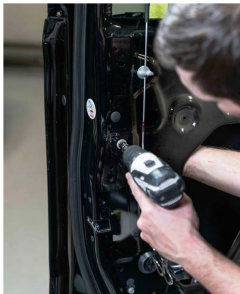
▲ Figure 67. Remove the upper window track bolt
