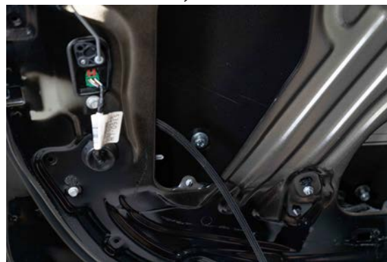
▲ Figure 56. The front, top crash bar bracket loosely installed
