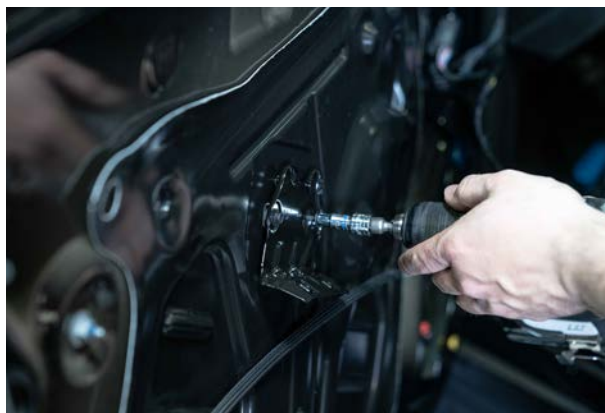
▲ Figure 32. Removing the door handle bracket
