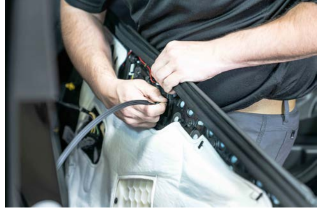
▲ Figure 30. Removing the door latch cable
