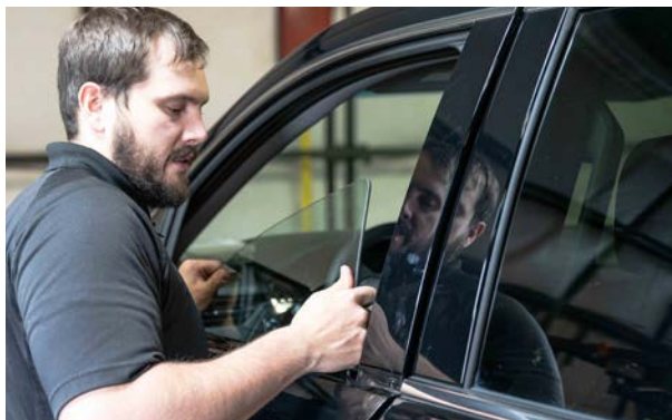
▲ Figure 36. Removing the window glass
