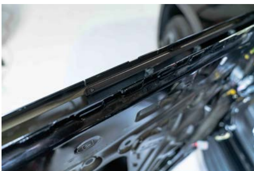
▲ Figure 59. Support Bracket aligned and installed
