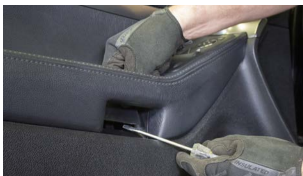
▲ Figure 25. Removing the armrest pocket trim cover
