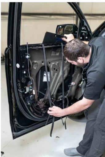
▲ Figure 54. Using the cradle created by the installation straps to lower the armor into the door.
