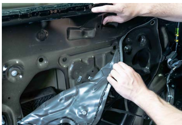
▲ Figure 33. Removing the weather seal
