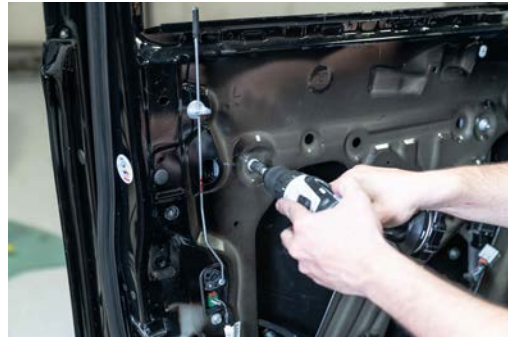
▲ Figure 64. Tightening the regulator mounting bolt
