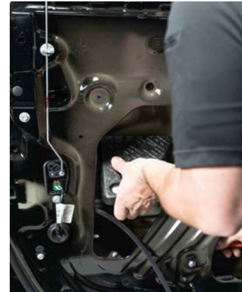
▲ Figure 45. Prying out the foam block
