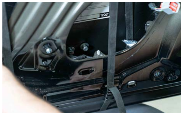
▲ Figure 55. The front, top of the crash bar bracket loosely installed
