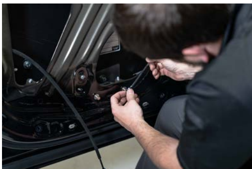
▲ Figure 65. Installing the lower mounting bracket
