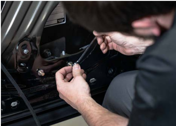
▲ Figure 49. Lower Mounting Bracket loosely installed
