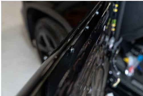
▲ Figure 57. Loosely installed upper mounting bracket
