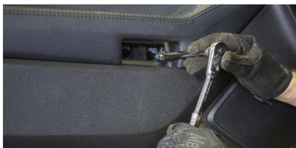
▲ Figure 26. Removing the armrest pocket bolts
