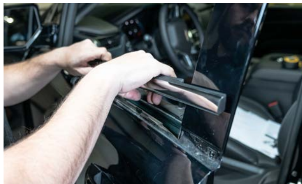
▲ Figure 24. Removing the outer window weatherstrip
