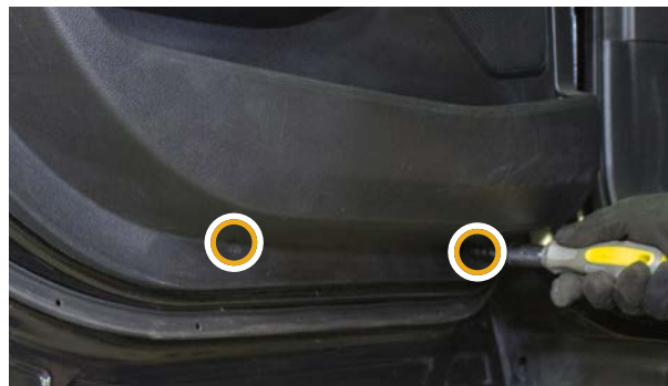
▲ Figure 27. Removing the door panel bolts
