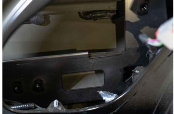
▲ Figure 50. Crash Bar Mounting Bracket placed on crash bar
