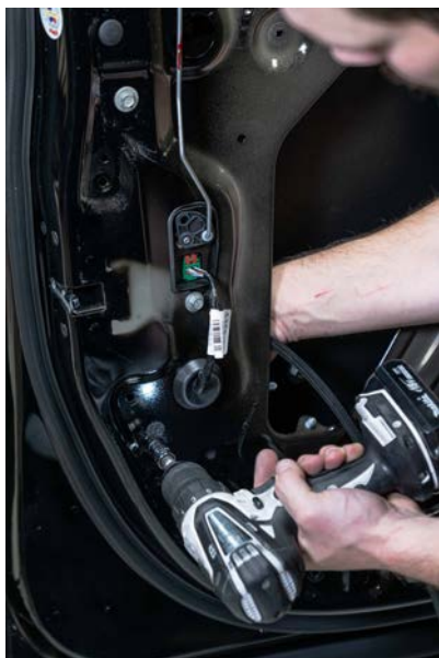
▲ Figure 68. Loosening the rear window track
