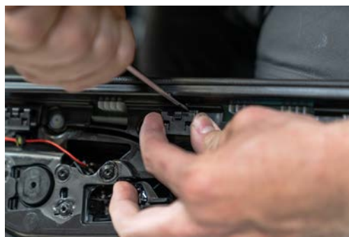
▲ Figure 70. Removing the metal clip from the interior panel
