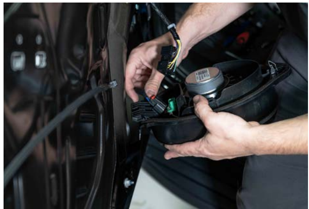
▲ Figure 31. Disconnecting the speaker harness
