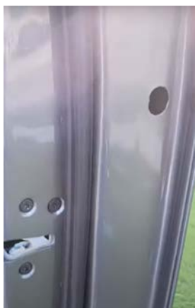
▲ Figure 59. Showing the two nuts on exterior door handle
