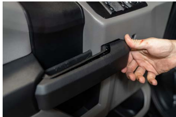
▲ Figure 22. Removing the handle panel
