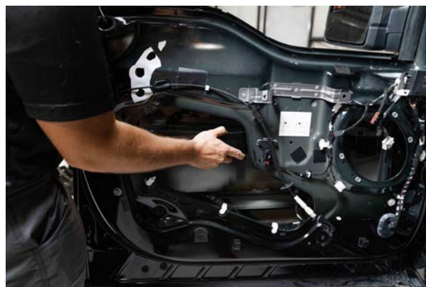
▲ Figure 62. Dry fitting the upper bracket into the door
