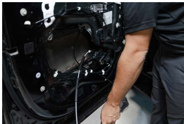
▲ Figure 44. Removing window regulator
