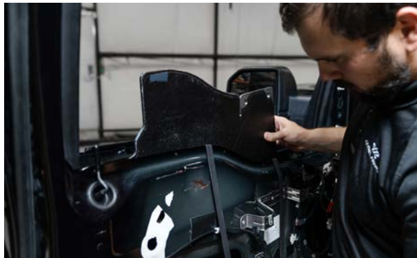
▲ Figure 76. Placing the armor into the door
