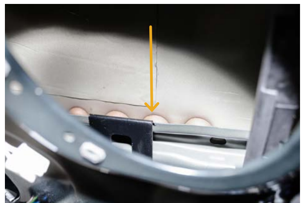
▲ Figure 72. Crash bar bracket and located in the door
