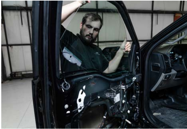
▲ Figure 37. Removing the window glass
