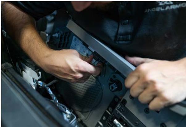
▲ Figure 27. Removing the door panel
