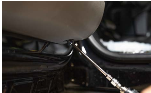
▲ Figure 25. Removing the lower panel bolts
