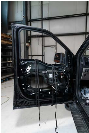
▲ Figure 74. Crash bar bracket and located in the door
