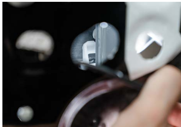
▲ Figure 34. Locating the window regulator clips
