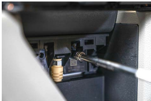
▲ Figure 24. Removing the interior door handle bolts
