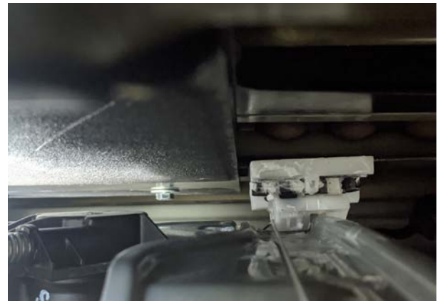
▲ Figure 82. Front window regulator clearance
