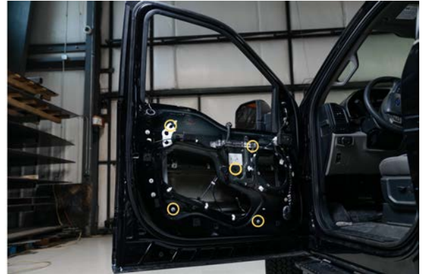
▲ Figure 39. Locating the hex nuts and bolt
