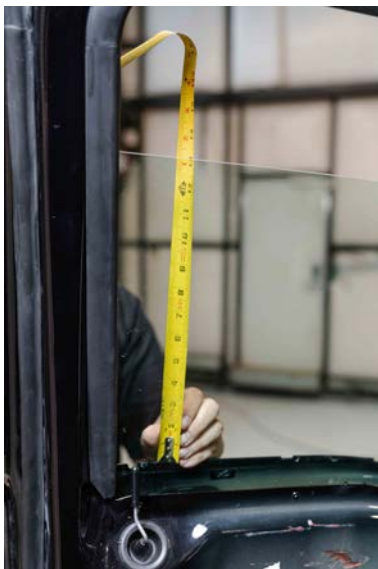
▲ Figure 32. Setting window height to 13 inches
