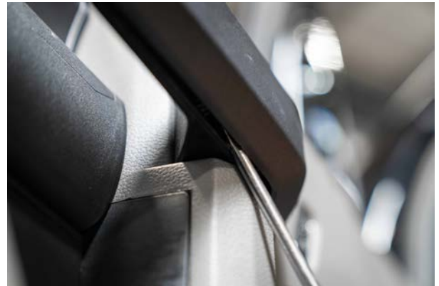
▲ Figure 21. Prying the trim panel loose.
