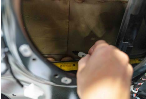
▲ Figure 70. Marking 9.25 inches toward the rear of the vehicle from the front of the crash bar.
