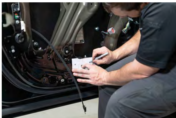
▲ Figure 46. Making the hole locations using the template provided (appended at the end of this guide)
