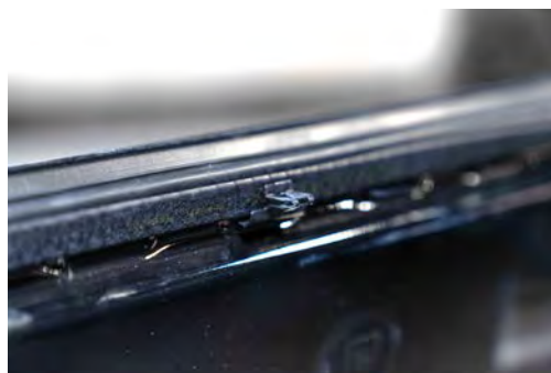
▲ Figure 71. Metal clip reinstalled to the door with the weatherstrip over the top
