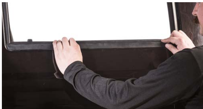
▲ Figure 20. Pressing down the window weatherstrip
