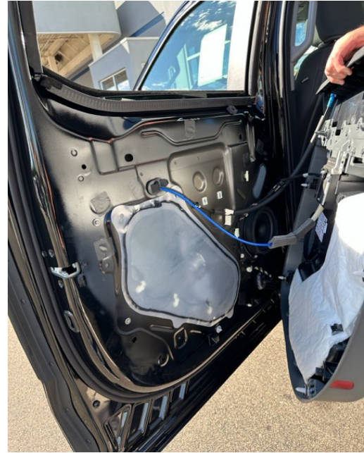
▲ Figure 19. Aligning and snapping the upper edge of the door panel on the interior portion of the door.
