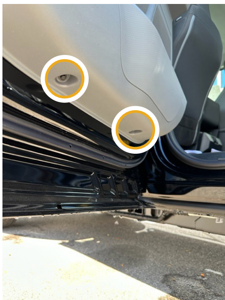
▲ Figure 8. Removing door compartment screws
