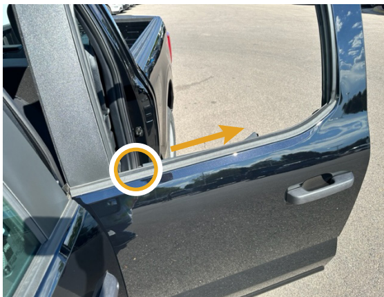
▲ Figure 14. Removing the window weatherstrip
