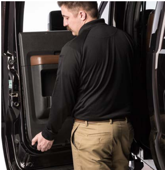
▲ Figure 11. Pulling door panel away from door.
