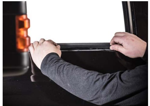
▲ Figure 18. Positioning the nylon folds over the window frame
