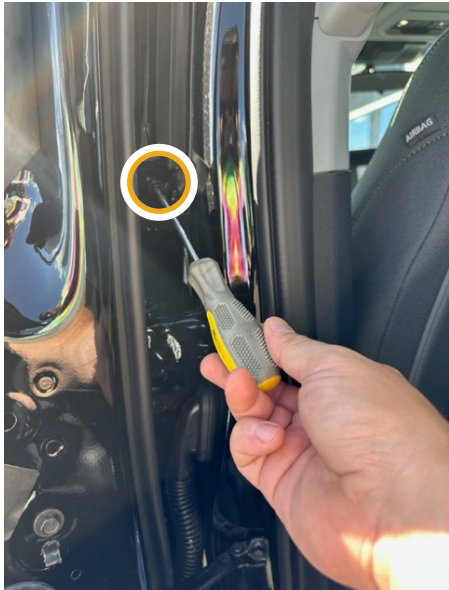
▲ Figure 13. Removing T-15 screw
