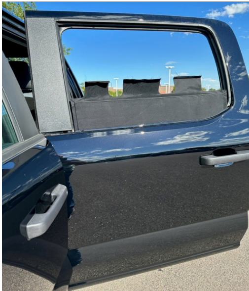
▲ Figure 16. Inserting the Ballistic Door Panel into the door
