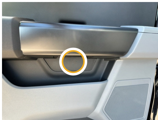
▲ Figure 9. Removing bolt cover
