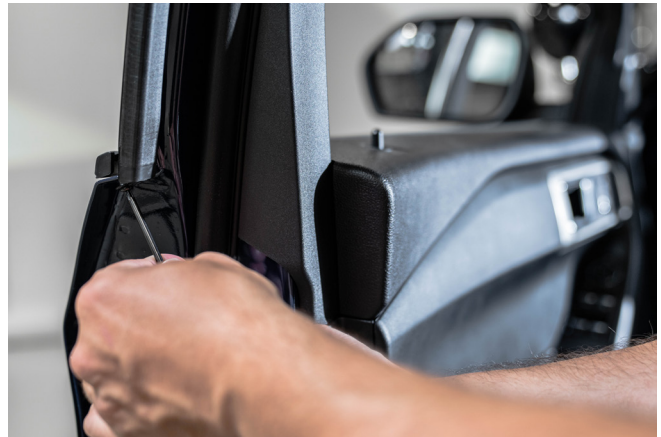
▲ Figure 5. Removing the Torx screw
