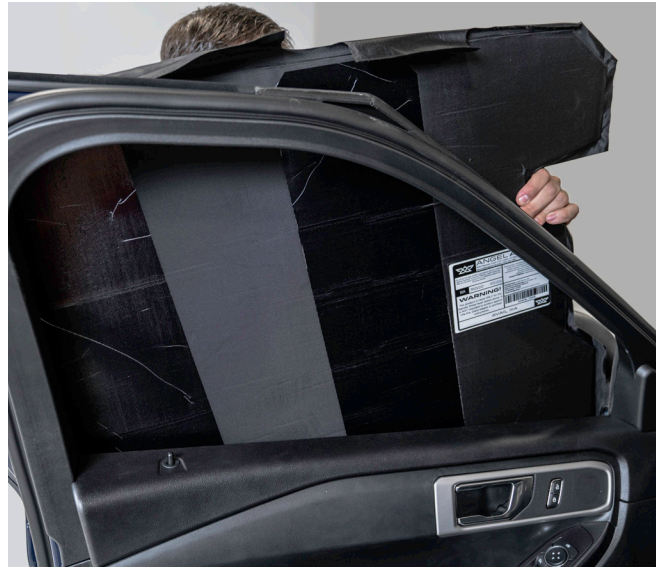
▲ Figure 7. Inserting the panel into the door
