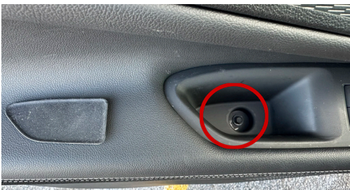
▲ Figure 23. Removing screw with 7mm socket
