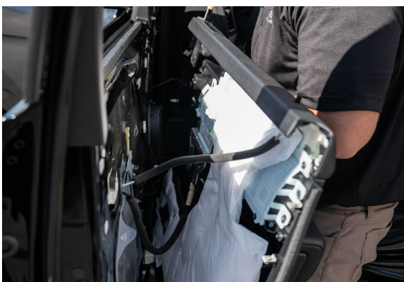
▲ Figure 17. Prying open the vehicle interior door trim panel
