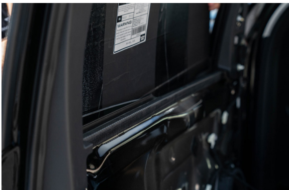
▲ Figure 24. Inserting panel into door
