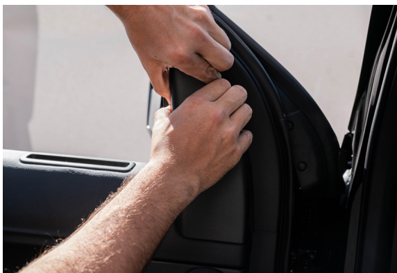
▲ Figure 15. Removing the trim cover
