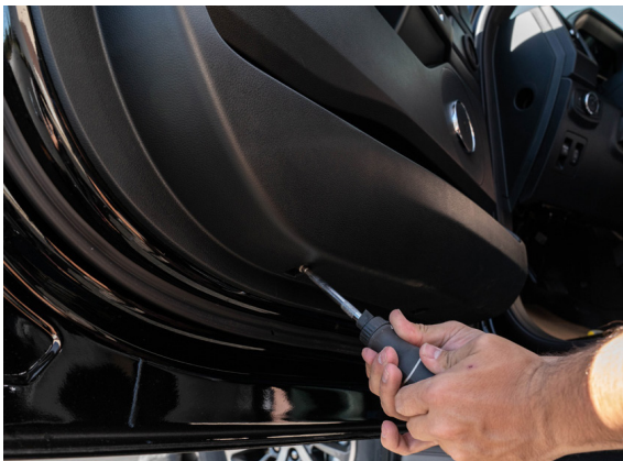
▲ Figure 12. Remove 7 mm panel mounting bolt
