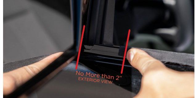
▲ Figure 27. Verifying the panel is no more than 2 inches from the front
