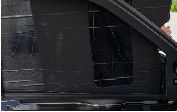
▲ Figure 23. Anti-abrasion panels facing the interior of the vehicle
