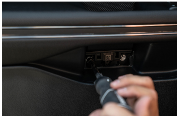
▲ Figure 14. Removing 8 mm panel mounting bolts
