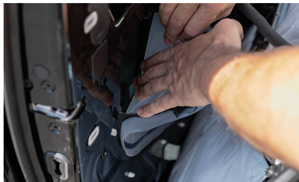
▲ Figure 18. Removing vapor barrier
