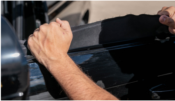
▲ Figure 26. Leaning back/pulling ballistic door panel toward exterior of the door.
