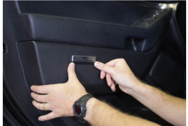
▲ Figure 30. Applying the brand label to the door
