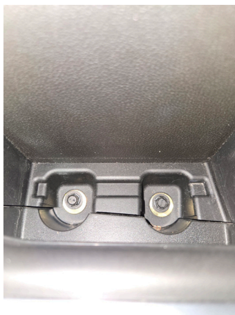
▲ Figure 24. Bolts revealed in handle pocket
