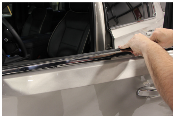
▲ Figure 16. Reinstalling outer window weatherstrip
