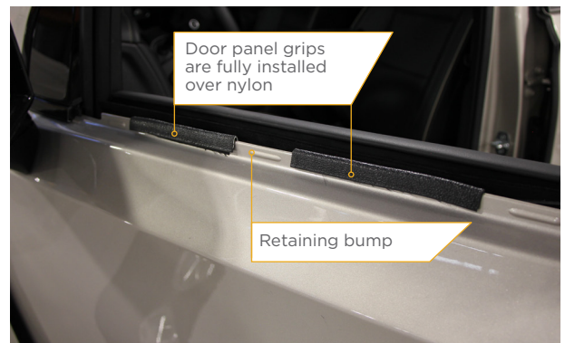
▲ Figure 15. Final placement of Door Panel Grips (presented on white door to show contrast)
