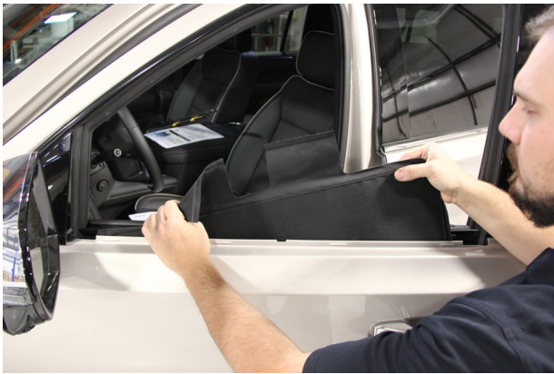
▲ Figure 11. Holding ballistic door panel against window glass while leaning back
