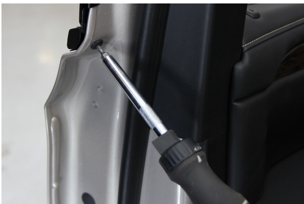
▲ Figure 8 Removing outer window weatherstrip screw
