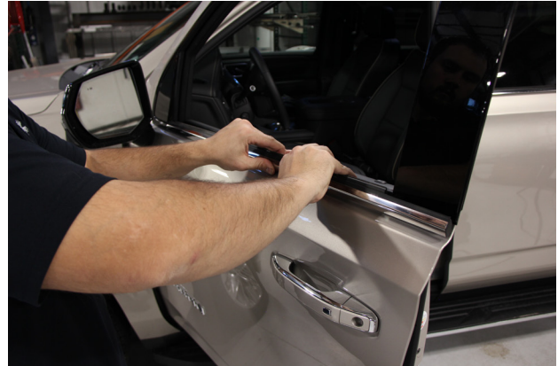
▲ Figure 9. Removing outer window weatherstrip
