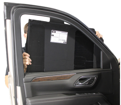
▲ Figure 10. Inserting ballistic panel into door with anti-abrasion panels facing vehicle interior
