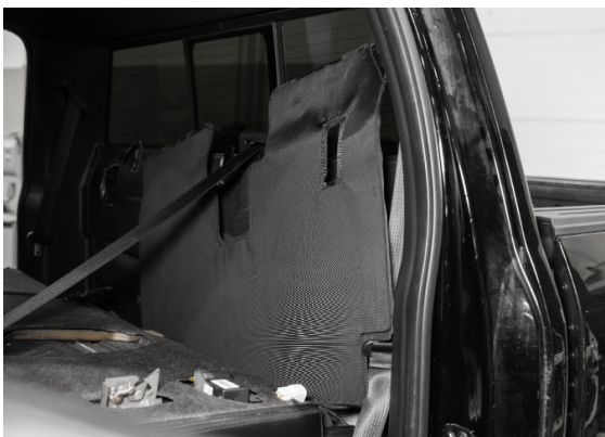
▲ Figure 4. Inserting driver side panel
