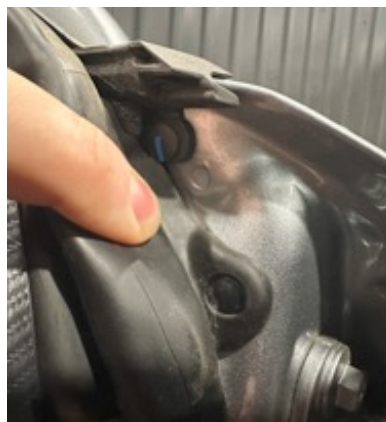
▲ Figure 25. Removing the front edge of plastic rivet from exterior window trim
