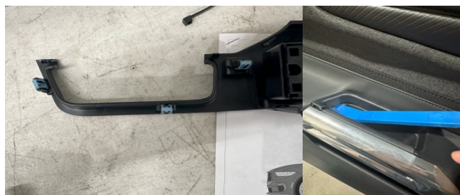
▲ Figure 16. Removing door control from handle edge
