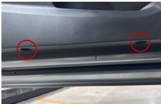
▲ Figure 18. Locations of 7mm screws
