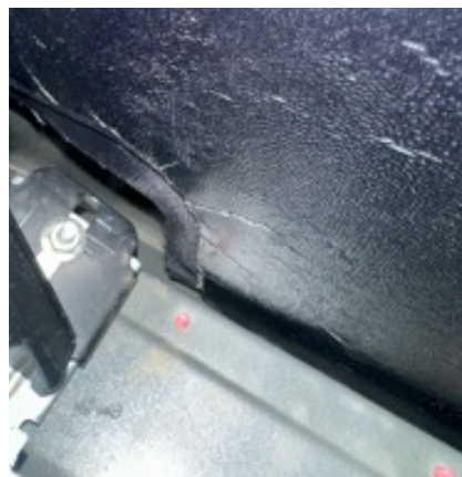
▲ Figure 28. Space between armor and window regulator
