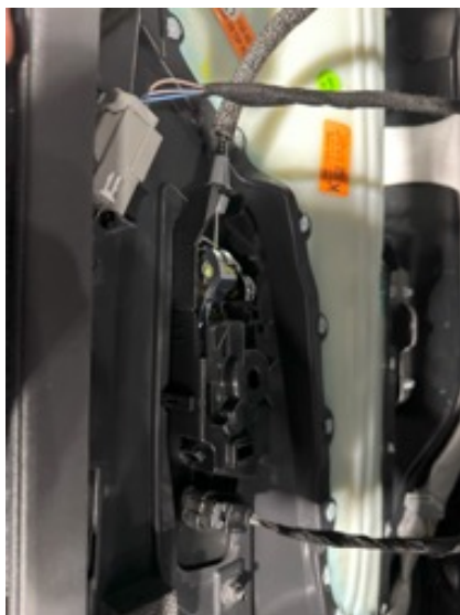
▲ Figure 19. Door handle cable and wiring harnesses
