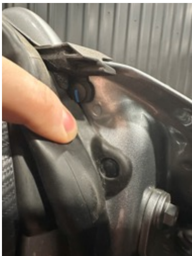
▲ Figure 22. Plastic rivets on window triangle rubber seal
