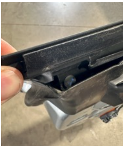
▲ Figure 26. Hidden plastic rivet
