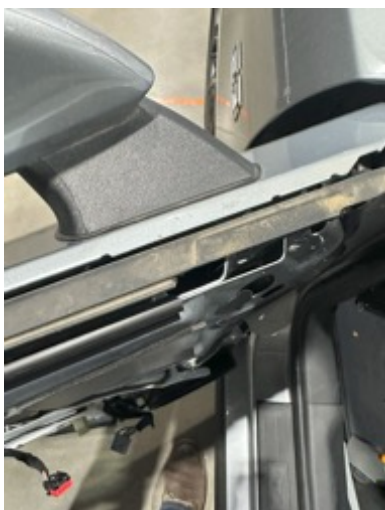
▲ Figure 23. Removing the window triangle
