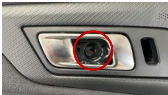
▲ Figure 15. Location of handle bolt
