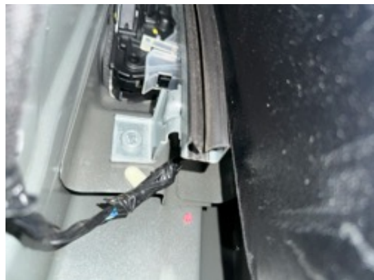
▲ Figure 27. Rear of armor behind rear window track
