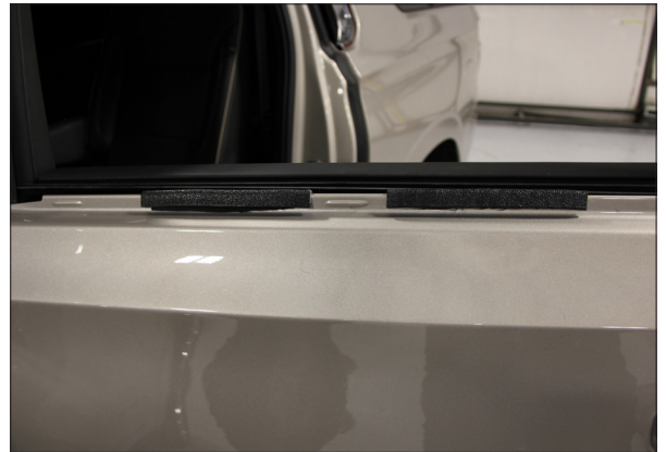
▲ Figure 15. Proper placement of Door Panel Grips
