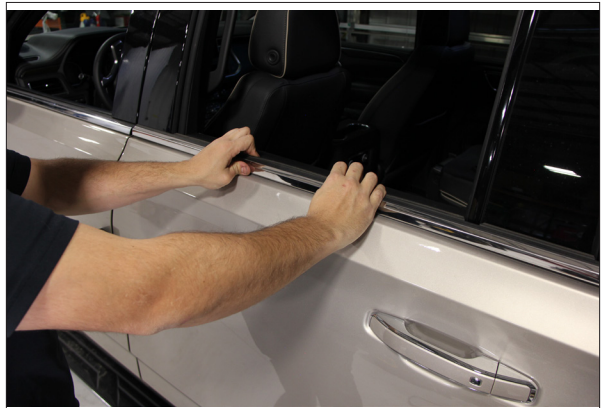
▲ Figure 10. Removing the weatherstrip
