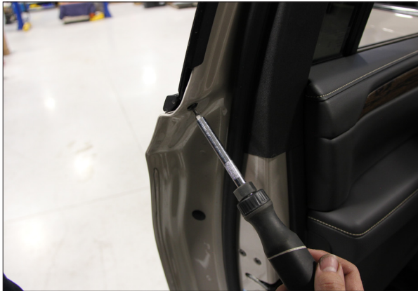
▲ Figure 7. Removing the rear Torx screw
