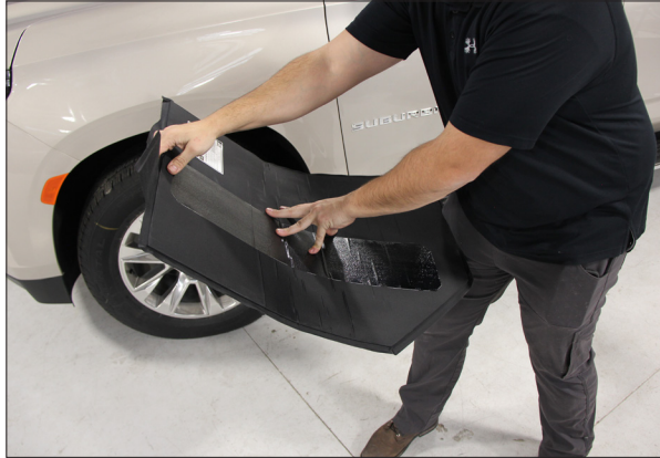
▲ Figure 11. Bending the Ballistic Door Panel to create a slight curve
