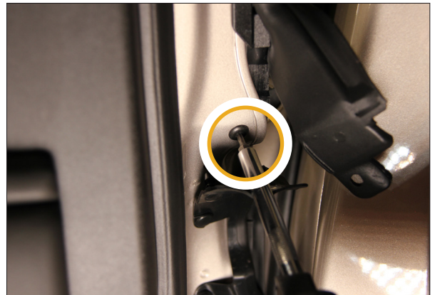
▲ Figure 9. Exposing the front Torx screw
