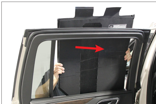
▲ Figure 12. Pushing panel forward while inserting panel
