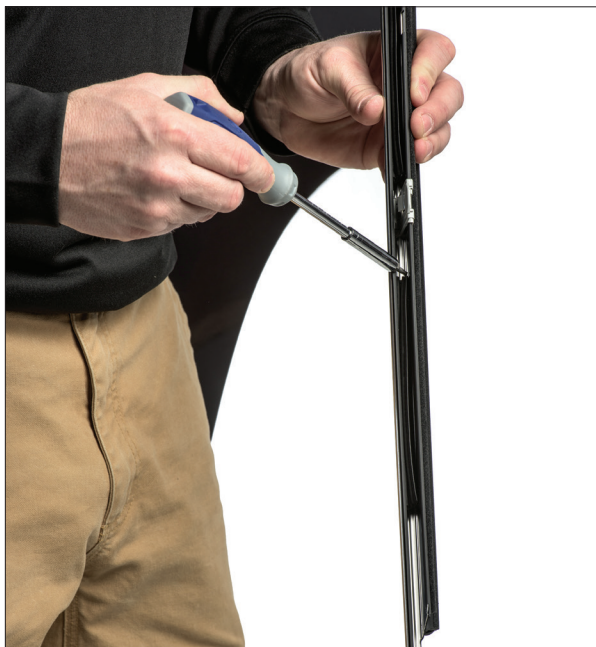
▲ Figure 19. Removing two Door Panel Grips from inside the weatherstrip
