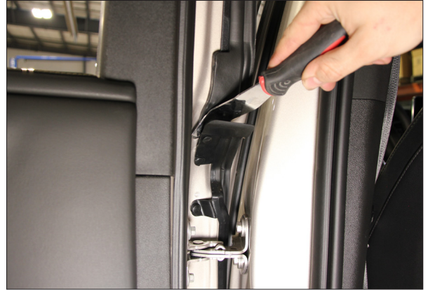
▲ Figure 8. Exposing the front Torx screw
