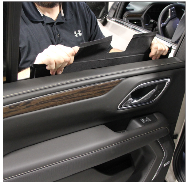
▲ Figure 13. Sliding panel down into the door
