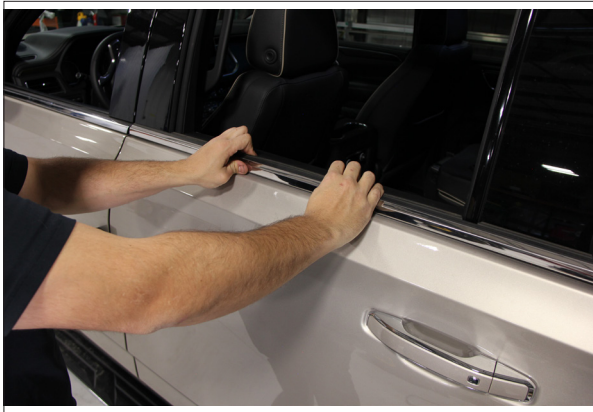
▲ Figure 16. Proper weatherstrip alignment
