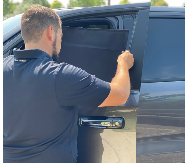
▲ Figure 24. Inserting panel between window glass and outer door skin
