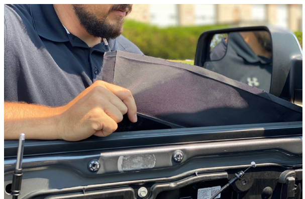
▲ Figure 25. Sliding panel towards front of door frame
