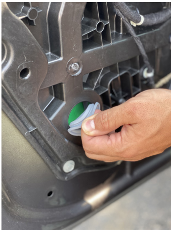
▲ Figure 18. Peeling back the moisture barrier to expose the window regulator bolt
