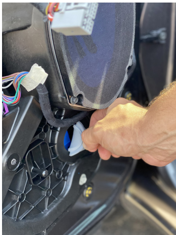
▲ Figure 19. Peeling back the moisture barrier to expose the window regulator bolt
