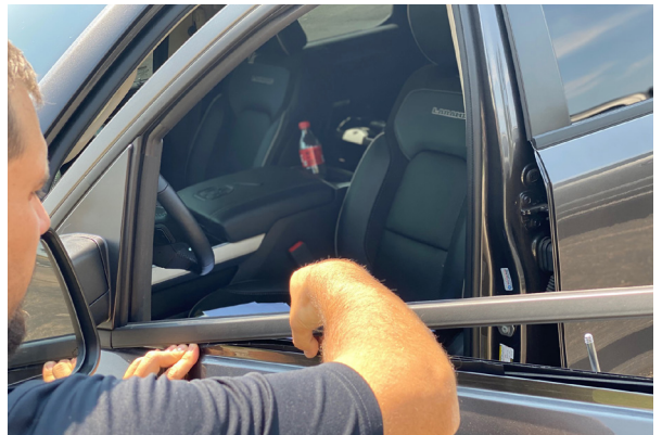
▲ Figure 28. Seating weatherstrip along window frame
