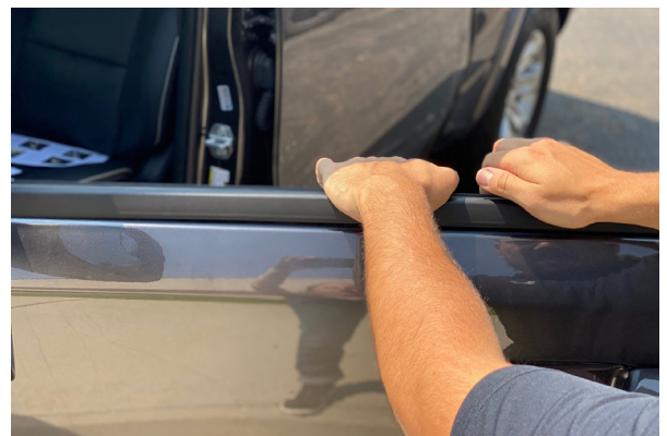
▲ Figure 29. Properly seated window weatherstrip
