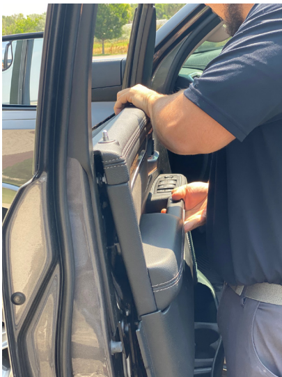
▲ Figure 15. Pulling the vehicle door panel away from door
