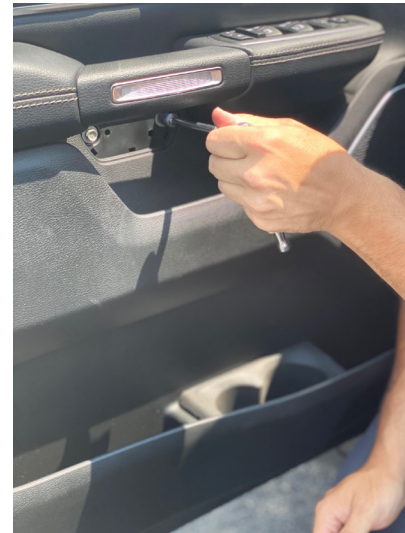
▲ Figure 13. Removing bolts from arm rest
