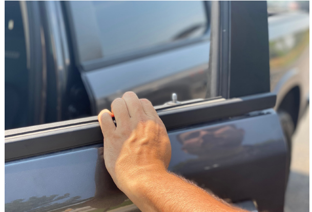
▲ Figure 10. Sliding back the outer window weatherstrip
