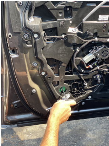
▲ Figure 21. Replacing the front window regulator bolt through the window regulator bolt access hole
