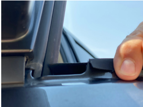
▲ Figure 26. Nylon fold is properly positioned on downward curve of the door seam
