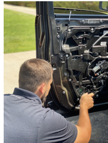
▲ Figure 20. Replacing the factory-installed window regulator bolt located behind the moisture barrier with the supplied replacement bolt
