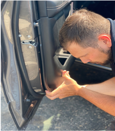
▲ Figure 14. Prying open the vehicle interior door trim panel
