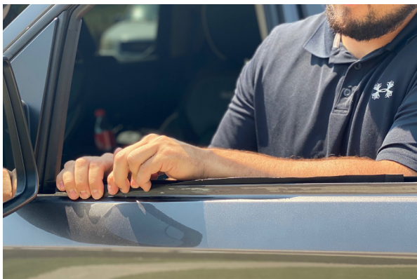
▲ Figure 27. Proper location of nylon fold
