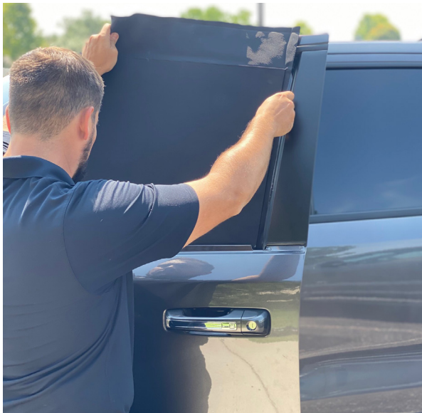
▲ Figure 23. Inserting panel between window glass and outer door skin
