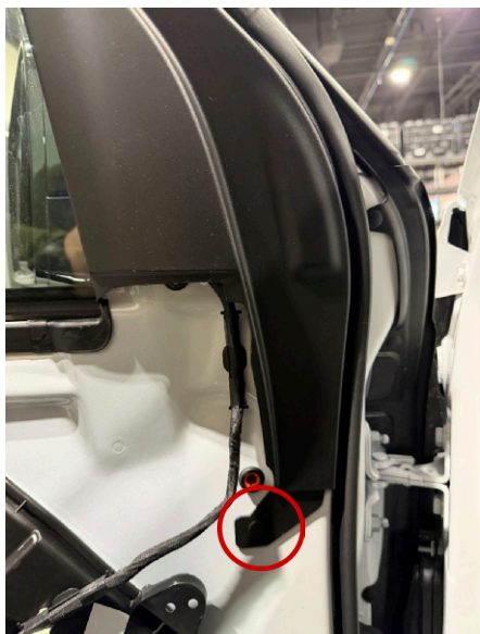
▲ Figure 18. Pulling front section away from the door
