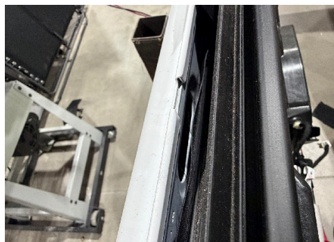
▲ Figure 27. Armor location under top oval cutouts in door cavity
