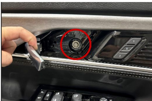
▲ Figure 14. Door handle bolt
