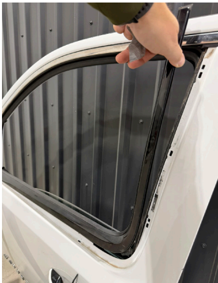
▲ Figure 21. Removing exterior trim from window
