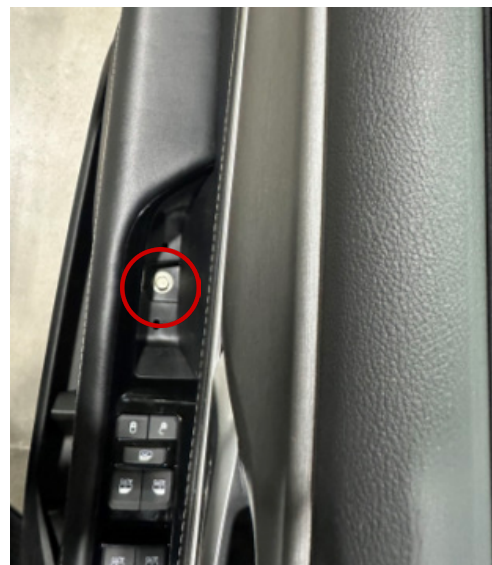
▲ Figure 16. Armrest pocket bolt
