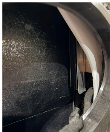
▲ Figure 26. Armor location behind front window track
