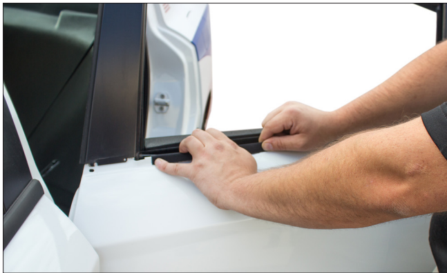
▲ Figure 18. Verifying the panel is \frac{3}{4} - 1 inch from the front of the window frame
