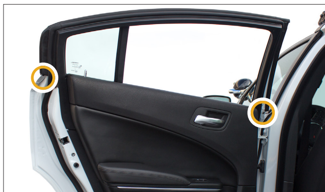
▲ Figure 8. Outer window weatherstrip screws
