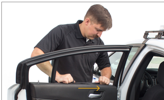
▲ Figure 17. Sliding Ballistic Door Panel forward
