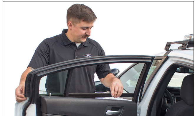
▲ Figure 20. Replacing the window weatherstrip
