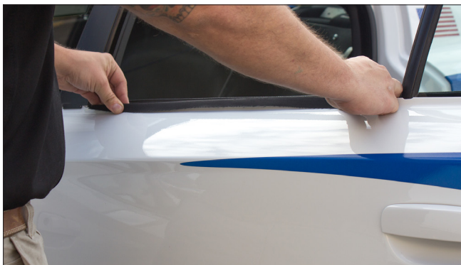
▲ Figure 16. Proper position of nylon folds when Ballistic Door Panel is slid all the way down
