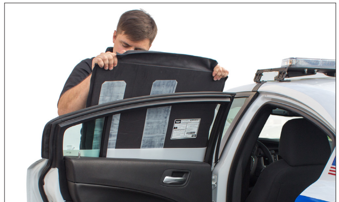
▲ Figure 13. Inserting Ballistic Door Panel
