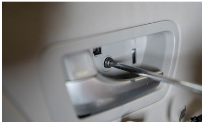
▲ Figure 12. Removing screw behind door handle
