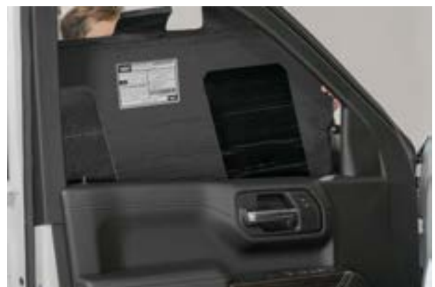
▲ Figure 10. Inserting ballistic panel into door with anti-abrasion panels facing vehicle interior
