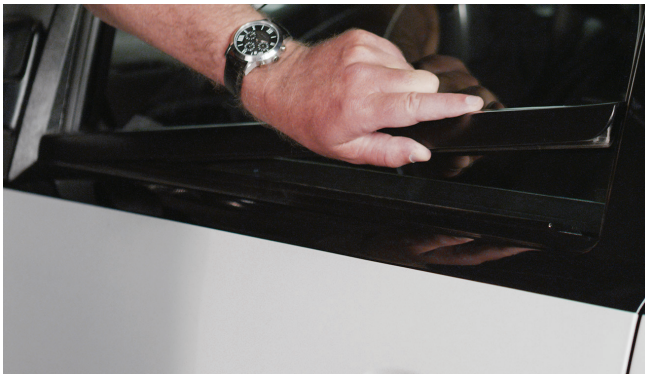
▲ Figure 11. Removing the outer window weatherstrip
