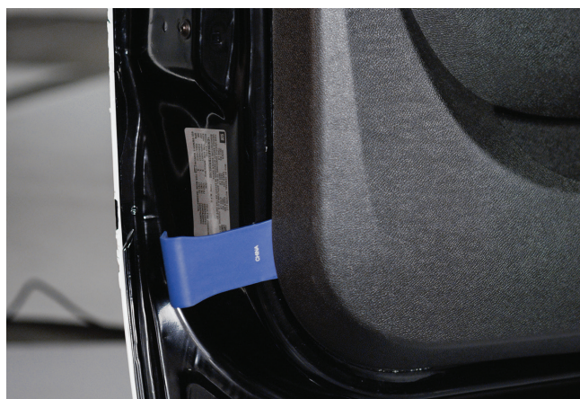
▲ Figure 8. Prying open the vehicle interior door panel
