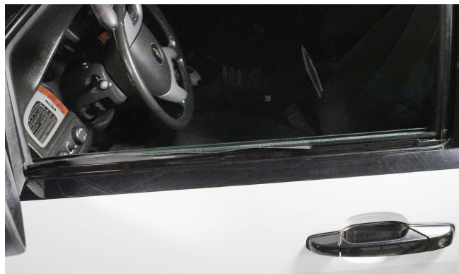
▲ Figure 15. Proper alignment of fold with window frame
