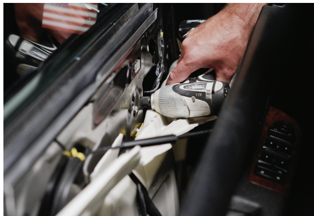
▲ Figure 10. Replacing the 10 mm factory-installed window regulator bolt with the supplied shorter 10 mm replacement bolt
