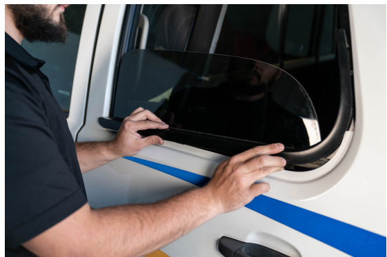
▲ Figure 16. Exterior view of properly installed ballistic panel
