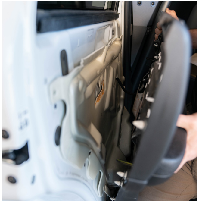
▲ Figure 8. Leaning open the interior door trim panel
