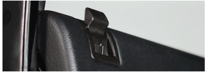
▲ Figure 17. Closed retaining panel on lock knob
