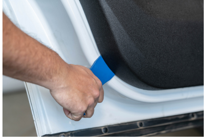
▲ Figure 7. Prying open the vehicle interior door panel
