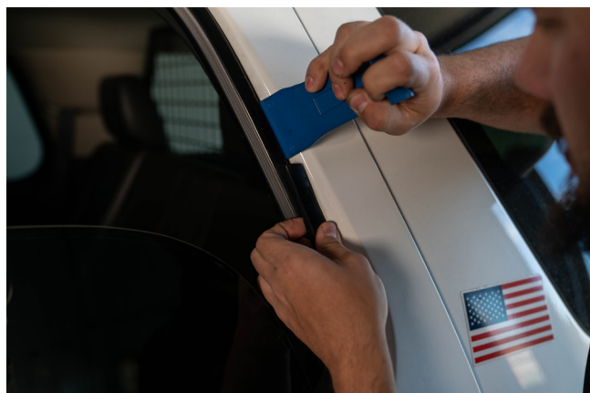
▲ Figure 11. Inserting the Angel Armor Ballistic Door Panel into the door
