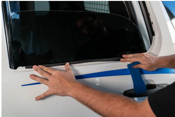
▲ Figure 15. Proper alignment of fold with window frame
