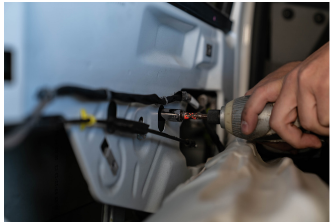
▲ Figure 9. Replacing the 10 mm factory-installed window regulator bolt with the supplied shorter 10 mm replacement bolt
