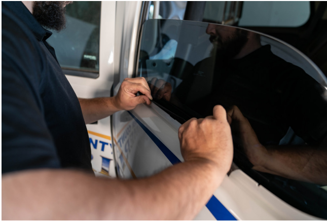
▲ Figure 13. Gripping ballistic door panel's top-edge nylon fold
