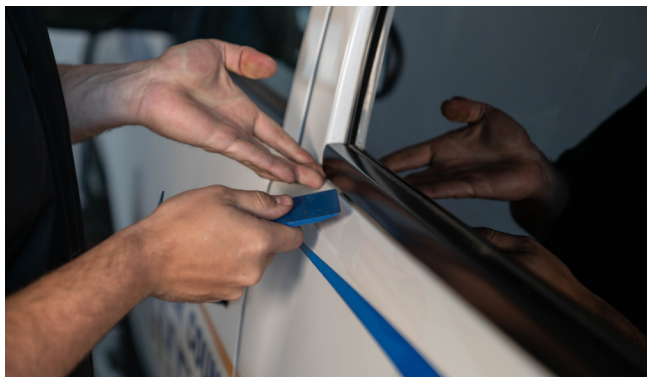
▲ Figure 10. Removing the outer window weatherstrip
