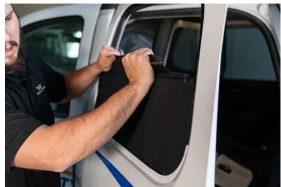
▲ Figure 12. Inserting the Angel Armor Ballistic Door Panel into the door
