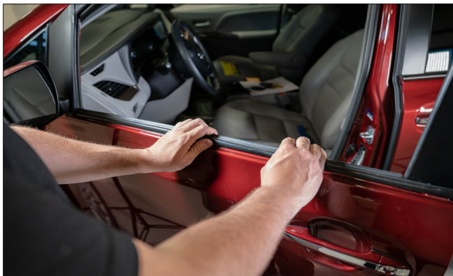
▲ Figure 23. Replacing the window weatherstrip
