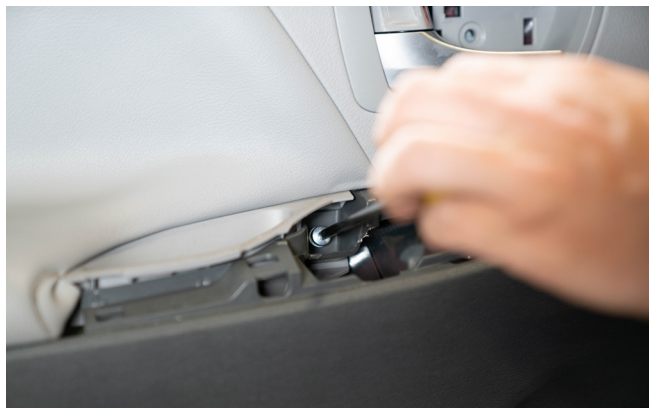
▲ Figure 13. Removing the screw behind the control panel
