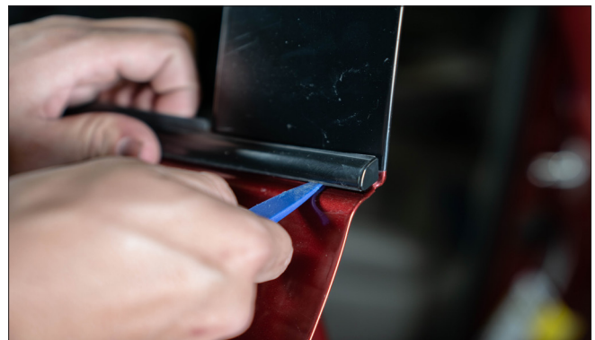
▲ Figure 9. Unhooking weatherstrip clip
