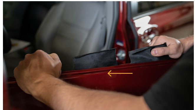
▲ Figure 18. Sliding ballistic door panel forward
