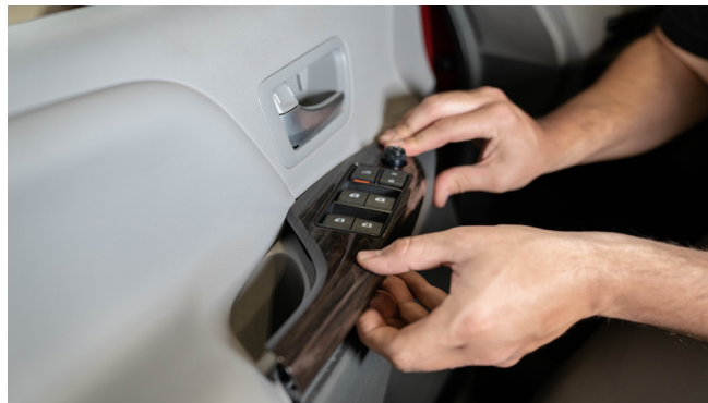
▲ Figure 12. Removing the control panel
