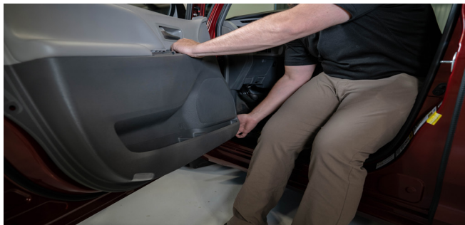
▲ Figure 14. Prying open the vehicle interior door trim panel
