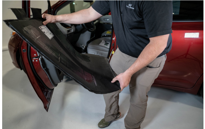
▲ Figure 15. Bending the ballistic door panel
