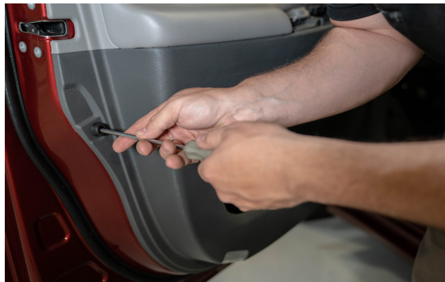
▲ Figure 11. Removing the back Phillips screw
