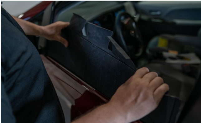
▲ Figure 16. Inserting ballistic door panel
