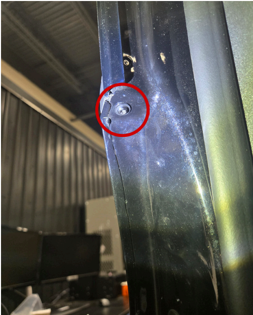
▲ Figure 10. Location of Torx screw holding outer window weatherstrip
