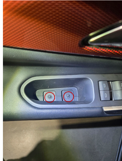
▲ Figure 11. Location of 7mm screws in the handle pocket
