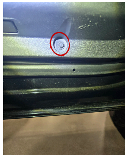
▲ Figure 12. Location of 7mm screw at the bottom of the trim panel
