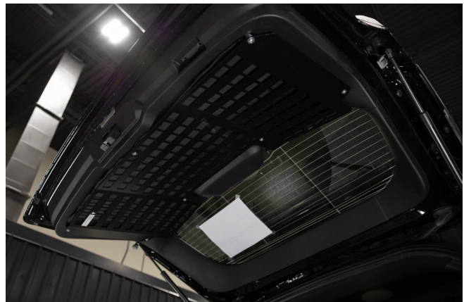
▲ Figure 40. Final armor placement once bolts are tightened
