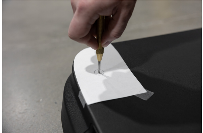
▲ Figure 29. Using drill guide template to center punch holes on the hatch interior
