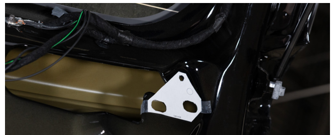
▲ Figure 35. Location of driver's side drill guide A
