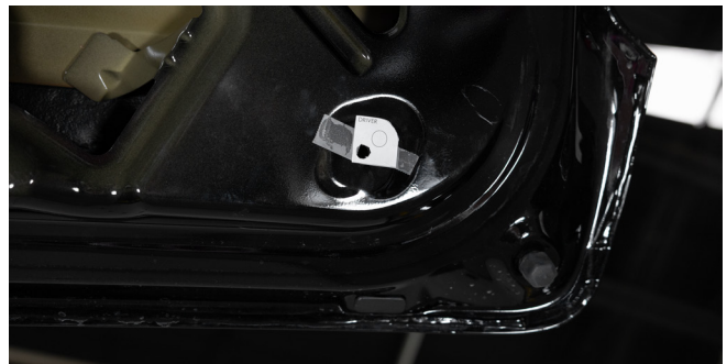
▲ Figure 36. Location of driver's side drill guide C
