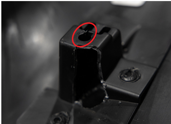
▲ Figure 32. Rivet housing after utility knife modifications
